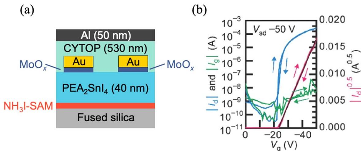
**Figure 26.** (PEA)<sub>2</sub>SnI<sub>4</sub> perovskite TFTs: (a) device structure and (b) transfer curves. [465] John Wiley & Sons. © 2016 WILEY-VCH Verlag GmbH & Co. KGaA, Weinheim.
