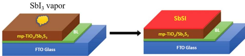
**Figure 22.** Configuration of SbSI-interlayered  $\text{Sb}_2\text{S}_3$  solar cell (the HTL is not shown). [205] John Wiley & Sons. © 2018 WILEY-VCH Verlag GmbH & Co. KGaA, Weinheim.
