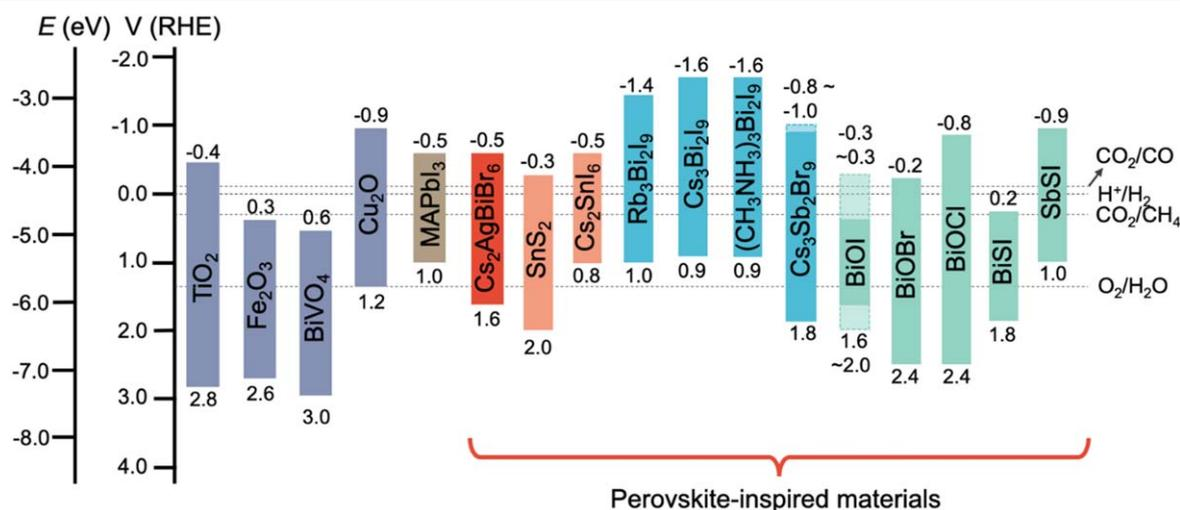
**Figure 24.** Band-edge positions of perovskite-inspired materials, which are compared to methylammonium lead iodide (MAPbI<sub>3</sub>) and traditional photocatalytic materials. The band positions are shown on a relative hydrogen electrode (RHE) potential scale (energy scale shown as a comparison). The RHE redox potentials of common half-reactions are given [406, 409]. The band positions are obtained from [133, 201, 237, 296, 394, 406, 409, 416–420].
