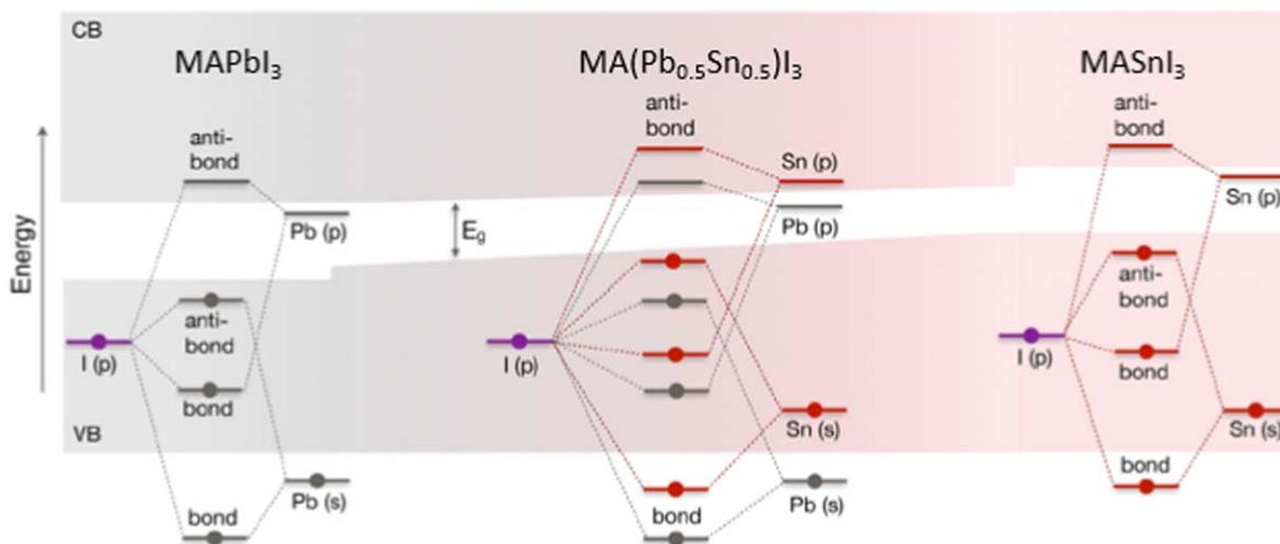
**Figure 15.** Schematic illustration of band gap bowing in  $\text{MA}(\text{Pb}_{1-x}\text{Sn}_x)\text{I}_3$  using a molecular orbital diagram to approximate the band structure of the crystal. Reprinted with permission from [227]. Copyright (2018) American Chemical Society.
