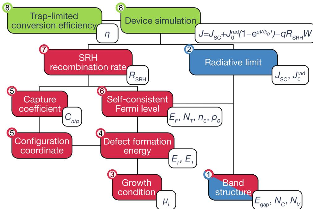
**Figure 3.** Schematic diagram of the calculation of the trap-limited conversion efficiency (TLC) metric. The dependent calculations are numbered and connected by lines, with the relevant calculated quantities appended. The red and blue boxes represent calculations for radiative and non-radiative electron–hole recombination, respectively. The combined device simulations are marked in green. Reproduced from [44]. CC BY 3.0.
