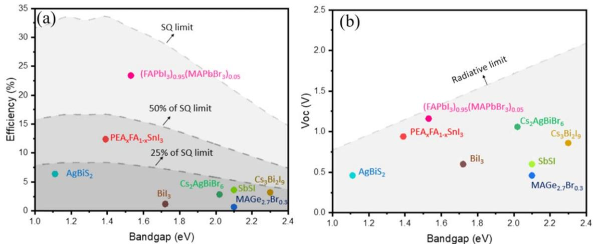
**Figure 23.** (a) The highest efficiencies and (b) the corresponding  $V_{OC}$  from various PIM-based PV devices reported in the literature to date. The highest values reported in Pb-based perovskite ( $(\text{FAPbI}_3)_{0.95}(\text{MAPbBr}_3)_{0.05}$ ) counterpart are also depicted.
