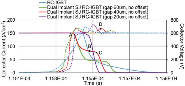
Fig. 6. Inductive load turn-off waveform for the Trench RC-IGBT and Trench Dual Implant SJ RC-IGBT with  $L_{gap}=60\mu\text{m}$ ,  $40\mu\text{m}$  and  $20\mu\text{m}$  (no offset), ambient temperature = 298K. Dashed lines voltage; solid line current.
