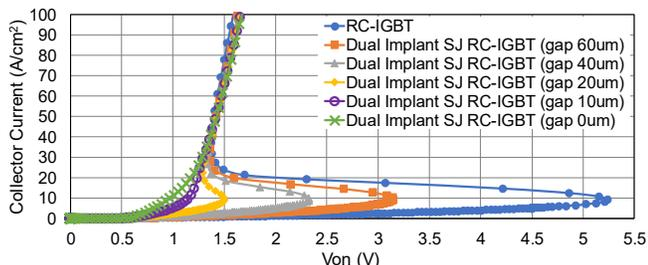
Fig. 3. On-state characteristics of Dual Implant SJ RC-IGBT, ambient temperature = 298K, SJ pillars have no offset between anode and cathode side
