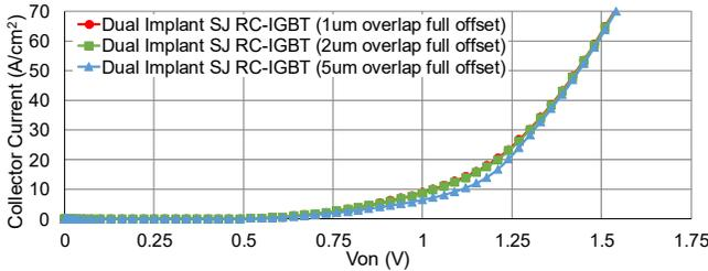
Fig. 5 On-state characteristics of Dual Implant SJ RC-IGBT with different amounts of overlap for full offset between anode and cathode SJ implants, ambient temperature = 298K
