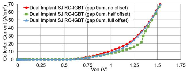
Fig. 4. On-state characteristics of Dual Implant Full SJ RC-IGBT with varying offset between anode and cathode SJ implants, ambient temperature = 298K
