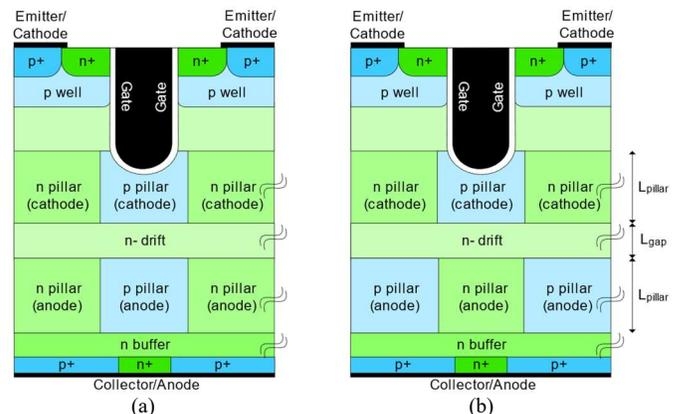
Fig. 1. Dual Implant SJ RC-IGBT structure (not to scale) (a) anode/cathode pillar with no offset, (b) anode/cathode pillar with full offset
