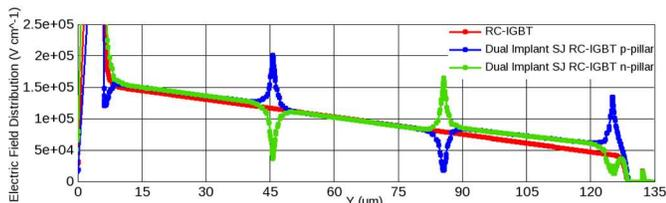
Fig. 2. Electric field distribution under blocking conditions (1.2kV) of the Trench RC-IGBT and Dual Implant Trench SJ RC-IGBT, thickness 135µm
