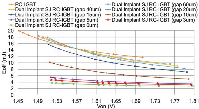
Fig. 7. Technology curves of Trench RC-IGBT and Dual Implant SJ RC-IGBT with varying  $L_{gap}$ , no offset,  $V_{on}$  at  $100\text{A}/\text{cm}^2$ , ambient temperature 298K
