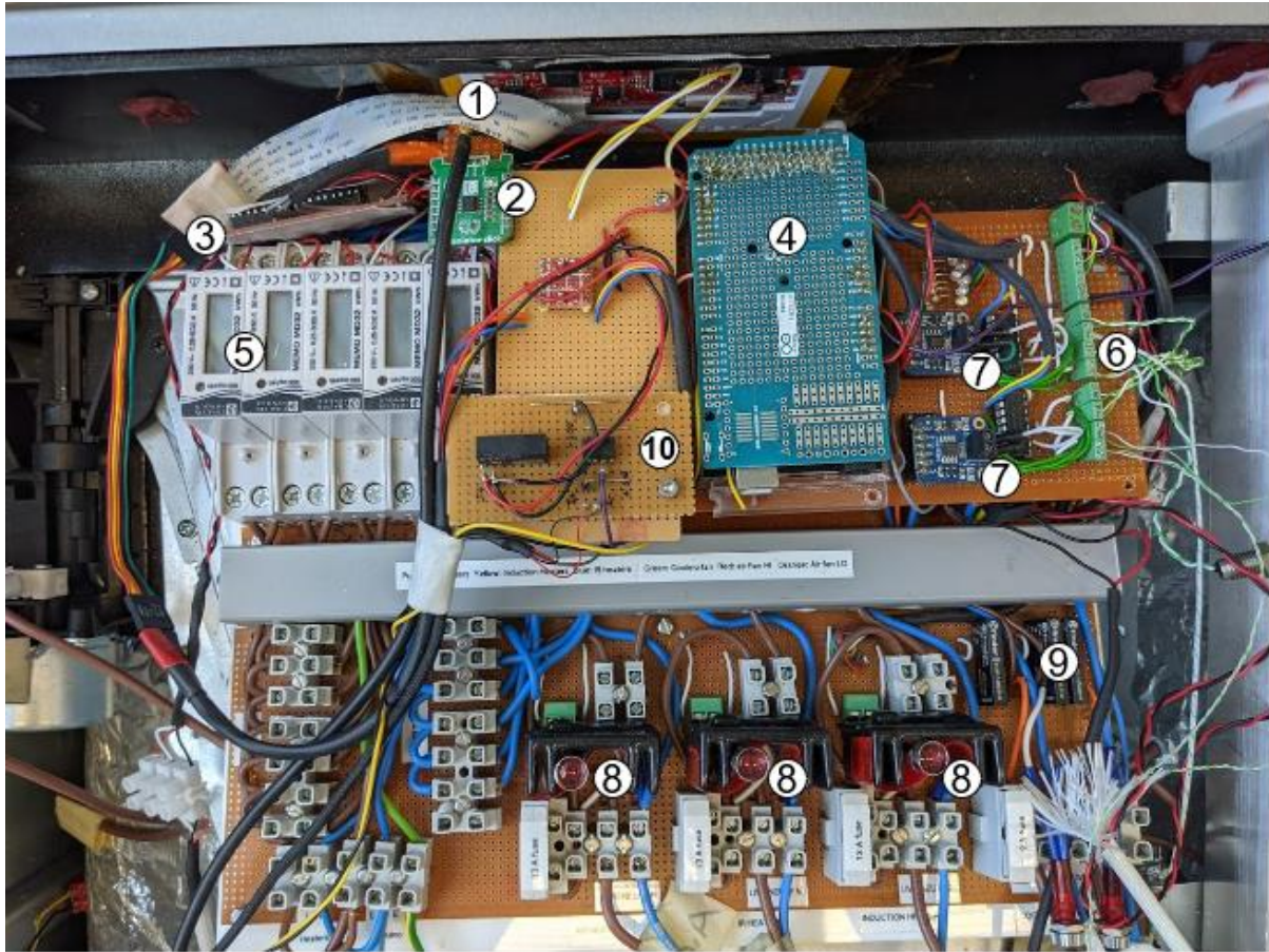
Figure 4.7: Labelled photograph of the control board for prototype II. 1 – Resistive touch screen, 2 – isolation chip for connection to the induction unit, 3 – optocoupler board connecting the power meters to the Arduino, 4 – Arduino MEGA microcontroller, 5 – power meters, 6 – thermocouple connections, 7 – multiplexors and thermocouple amplifiers, 8 – solid state relays for heater control, 9 – solid state relays for fan control.
