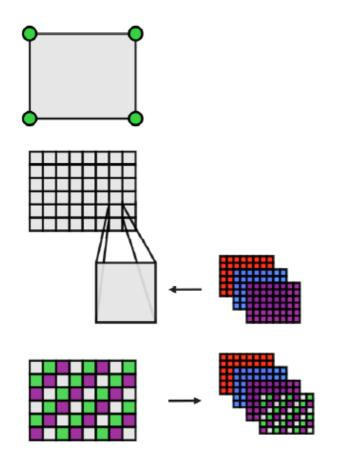
Application specifies geometry – GPU rasterizes
