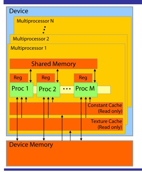
Divide 128 cores into 16 Multiprocessors (MPs)
