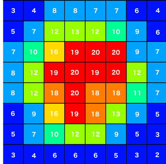
Figure 2.10: Occupancy (%) map for the 2-inch MAPMT. The EC was illuminated non-uniformly.
