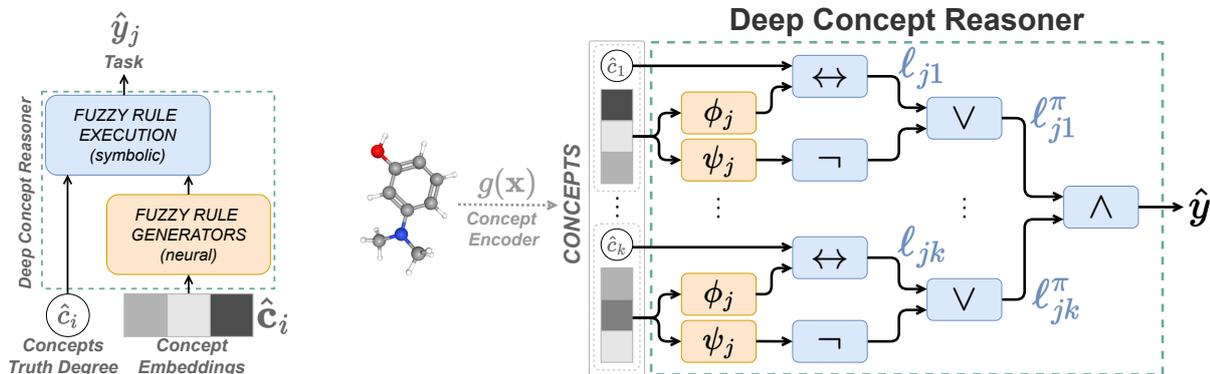
Figure 5.2: (left) Deep Concept Reasoner (DCR) generates fuzzy logic rules using neural models on concept embeddings. Then DCR executes the rule using the concept truth degrees to evaluate the rule symbolically. (right) Schema of DCR modules: first neural models  $\phi$  and  $\psi$  generate the rule, and then the rule is executed symbolically.
