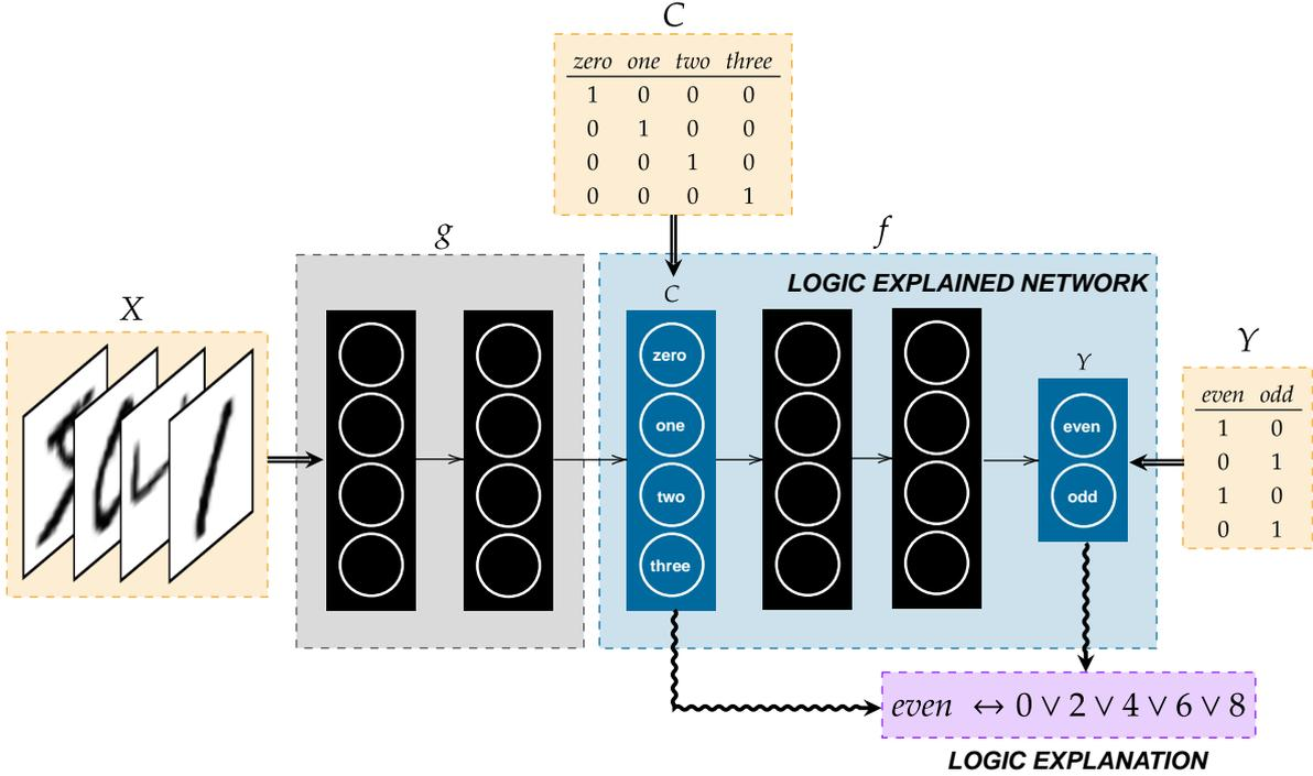
Figure 3.1: Logic Explained Network (LEN). The LEN is placed on top of a concept-encoder  $g$  which maps the input data into a first set of interpretable concepts. The figure shows a MNIST example: Handwritten digits are first classified by  $g$ . A LEN is then employed to classify and explain whether the digit is even or odd.
