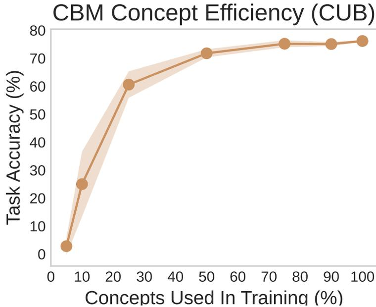
Figure 4.1: Real-world conditions (e.g., concept incompleteness and noisy supervisions) impair Concept Bottleneck Models (CBMs) task accuracy. As concept supervisions available for training are reduced, the task accuracy drops dramatically.
