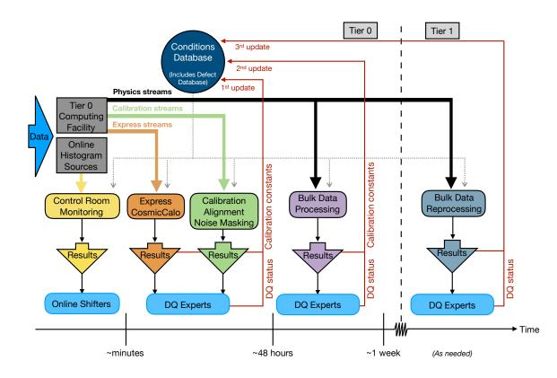
**Figure 2.** Schematic diagram illustrating the nominal Run 2 operations workflow for the data quality assessment of ATLAS data. Online histogram sources include the high-level trigger farm, the data acquisition system, and full reconstruction of a fraction of events accepted by the trigger.
