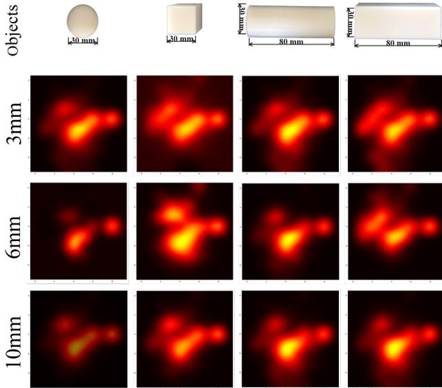
Fig. 6: 3D-printed Sphere, Cube, Half-Cylinder and Cuboid (view from above) and relative tactile images computed (averaged sensor readings over three trials).
