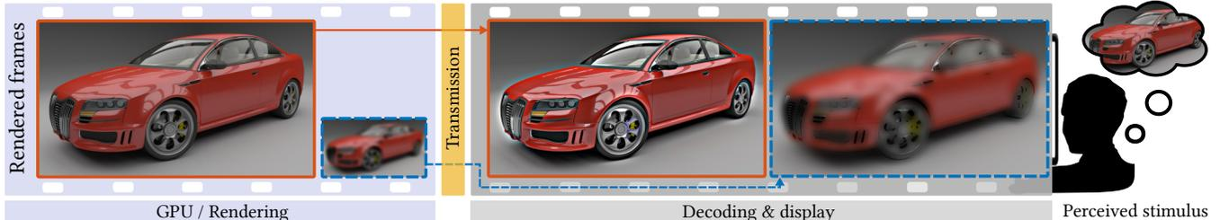
Figure 1: Our technique renders every second frame at a lower resolution to save on rendering time and data transmission bandwidth. Before the frames are displayed, the low resolution frames are upscaled and high-resolution frames are compensated for the lost information. When such a sequence is viewed at a high frame rate, the frames are perceived as though they were rendered at full resolution.
