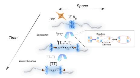
Figure 7. Schematic of the Spatial Separation of Triplet Pairs from the 2<sup>1</sup>A<sub>g</sub><sup>-</sup> State in pi-Conjugated Molecular Systems
