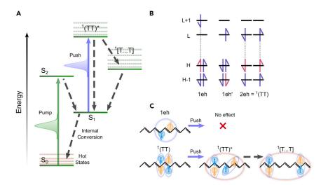
Figure 1. Energy Levels, Dynamics, and Electronic Properties of the Key Excited States of 1D pi-Conjugated Polymers of C₂H Molecular Symmetry
