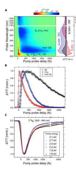
Figure 3. Transient Electronic Response of 3-BCMU Polydiacetylene following Photoexcitation
