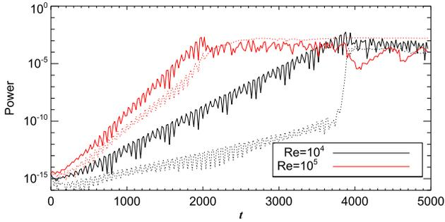
**Figure 2.** Largest spectral components of  $u_x$  (solid) and  $u_z$  (dashed) as a function of time for two values of  $Re$  ( $=10^4$  and  $10^5$ ). Both runs have  $R = 10^{-1.5}$  and  $Pe=4\pi^2$ .
