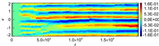
**Figure 15.** Space-time plot of  $u'_y$ , averaged over  $y$  and  $z$ , in  $t$ - $x$  showing the evolution of persistent zonal flows. Simulation parameters are  $R = 0.1$ ,  $Pe=4\pi^2$ ,  $Re=2 \times 10^5$  with  $L_x = 4L_z$ .
