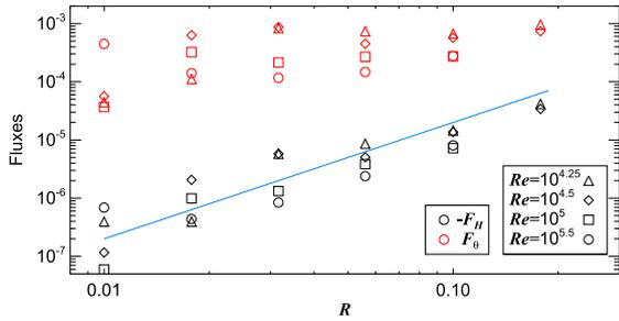
**Figure 17.** Turbulent fluxes,  $F_H = \langle u_x u'_y \rangle$  and  $F_\theta = \langle u_x \theta \rangle$ , as functions of  $R$  for  $Pe = 4\pi^2$ . The blue fitting line is given by  $2 \times 10^{-7} (R/0.01)^2$ .
