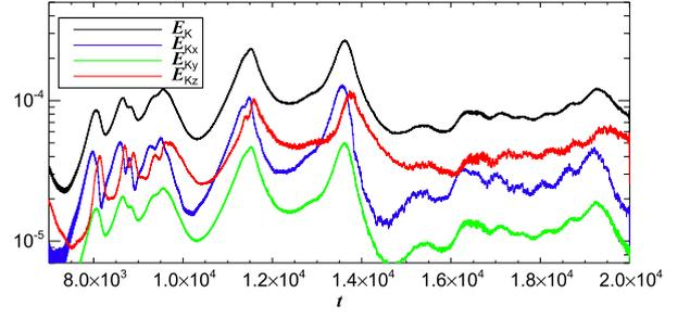
**Figure 6.** Kinetic energies as a function of time in a regime displaying non-linear waves and turbulence. The time series are filtered so that frequencies larger than 0.1 are removed. Simulation parameters are  $R = 0.01$ ,  $Pe=4\pi^2$ ,  $Re=10^{5.25}$ .
