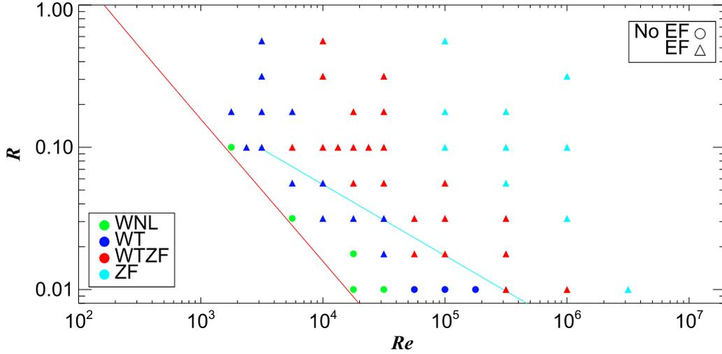
**Figure 16.** Plot depicting the different saturation routes open to the system in  $Re$ - $R$  space. The red line indicates marginal COS stability (when  $\lambda_{\text{crit}} = L$ ). The cyan line loosely denotes the boundary between pure wave turbulence and zonal flows and is given by  $R = 0.05 \times (Re/10^4)^{-1/2}$ .
