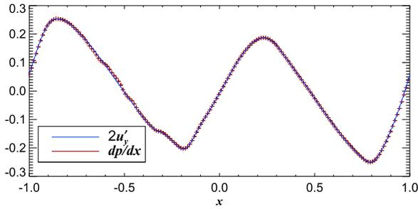
**Figure 13.**  $u'_y$  and  $dp/dx$  averaged over  $z$  at  $t = 9800$  (corresponding to the snapshots seen in panels 12d and 12h). Simulation parameters are  $R = 0.1$ ,  $Pe=4\pi^2$ ,  $Re=10^{5.5}$ .
