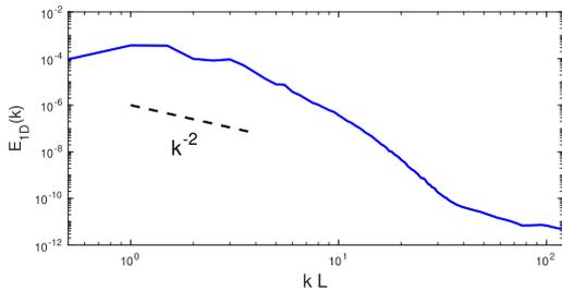
**Figure 8.** Power spectrum of kinetic energy as a function of wavenumber,  $k = \sqrt{k_x^2 + k_z^2}$  in the wave turbulent regime. Simulation parameters are  $R = 0.01$ ,  $Pe=4\pi^2$ ,  $Re=10^{5.25}$ .
