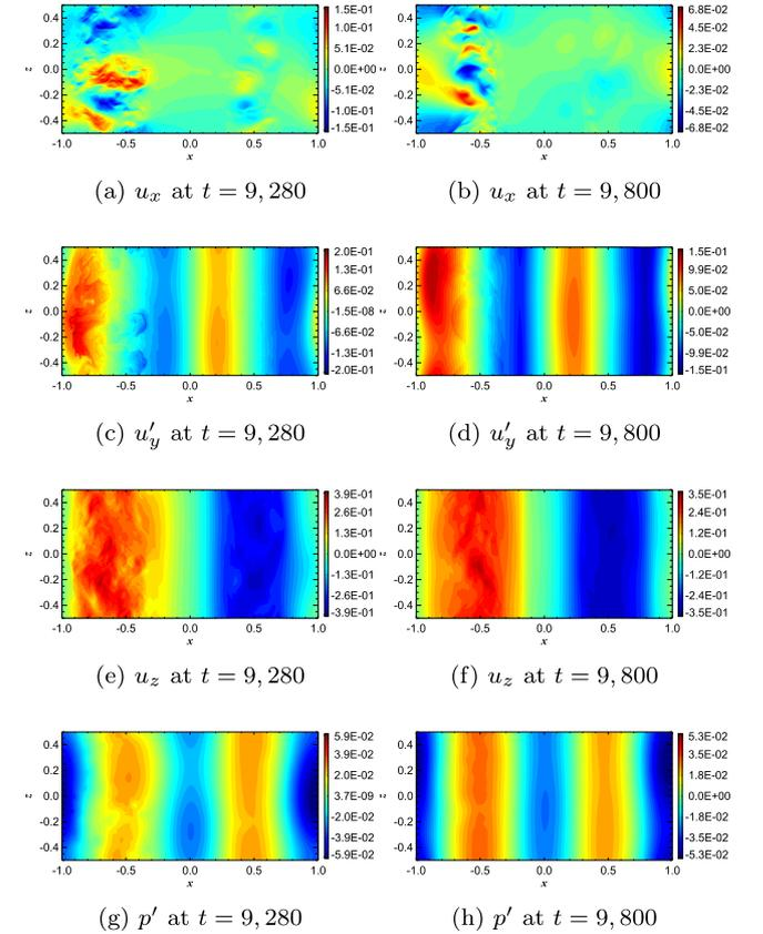
**Figure 12.** The perturbed velocity components and the perturbed pressure  $p'$  in  $x$ - $z$  space at two times for a run showing persistent zonal flows. Simulation parameters are  $R = 0.1$ ,  $Pe=4\pi^2$ ,  $Re=10^{5.5}$ .
