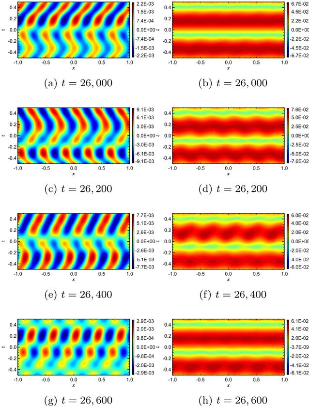
**Figure 5.** Plots of  $u_z$  (left-hand column) and  $u_A$  (right-hand column) in  $x$ - $z$  space at three times for a run saturating as the weakly non-linear regime. Simulation parameters are  $R = 10^{-1.5}$ ,  $Pe=4\pi^2$ ,  $Re=10^{3.75}$ .
