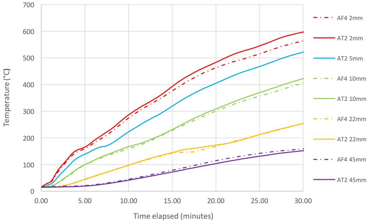
295 **Figure 8: Temperatures recorded in H-TRIS tests on AT2 and AF4 (simulated ISO 834 heating)**
