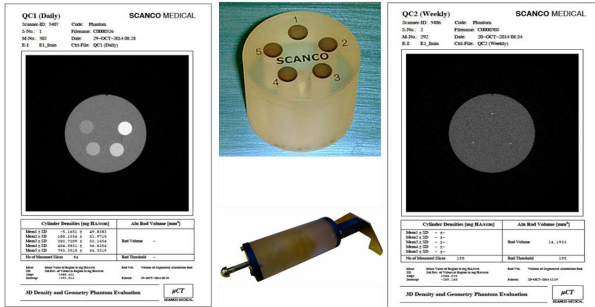
Figure 5.11 HR-pQCT calibration phantom scanned daily during the study period.
