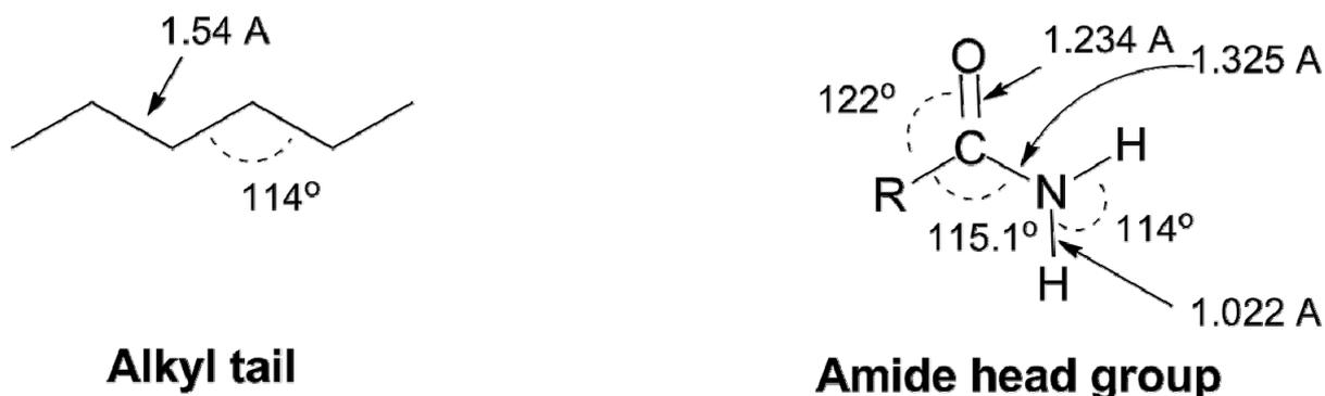
**Figure 4-6** Bond lengths and angles for generating an amide molecule for fitting
