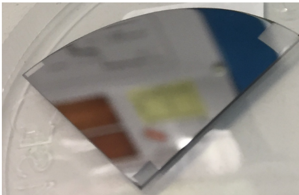
Figure 3.19 An image taken after the sample M2-0563 was taken out of the MBE chamber, showing a shiny like texture hinting towards a good quality growth. A sharp reflection can be observed on looking at the sample.
