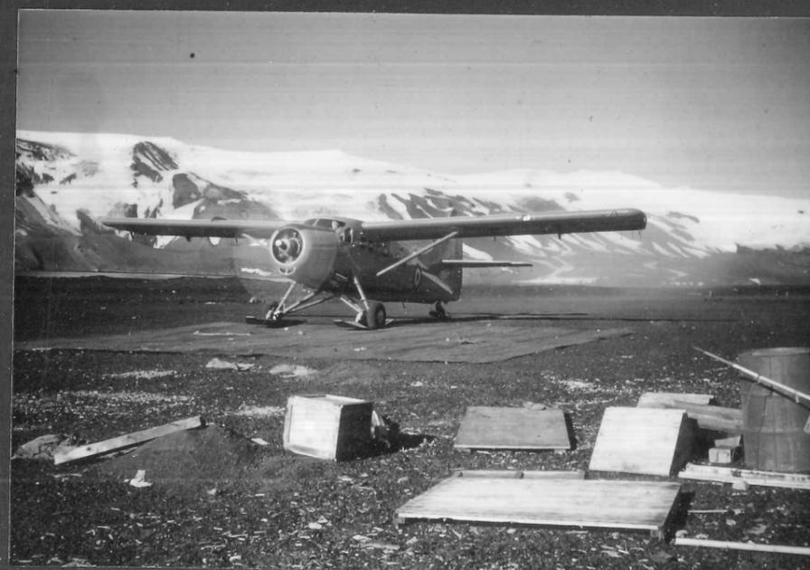
Plate 40. Test flying. Ski-wheel landing gear.
