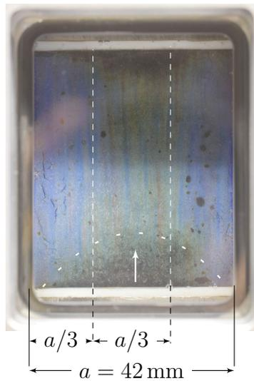
**Figure 5.21:** Thermochromic liquid crystal coated SS sample in bench-scale HEX observed through window. Onset of colour change in the middle third indicates a surface temperature of  $\sim 40^\circ\text{C}$ . White arrow indicates direction of flow and dashed curve illustrates a surface isotherm.
