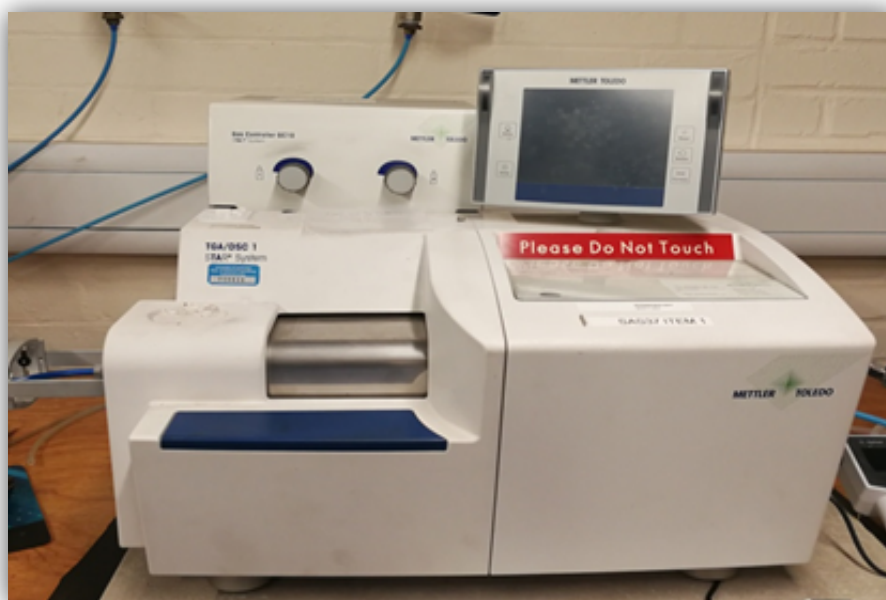
Figure 3.16 Mettler Toledo TGA/DSC connected to N 2 supply
