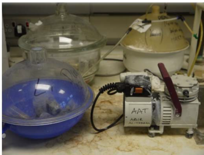
Figure 3.14 Vacuum drying chambers with a pump used to store samples
