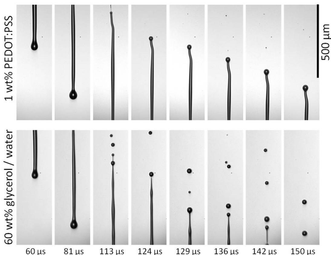
**Figure 2.** Jets formed at 65 V drive voltage by nominal 1 wt% PEDOT:PSS and G60W40 at the delay times shown. The nozzle exit was located just above the top edge of each image, and the jets were traveling vertically downwards.
