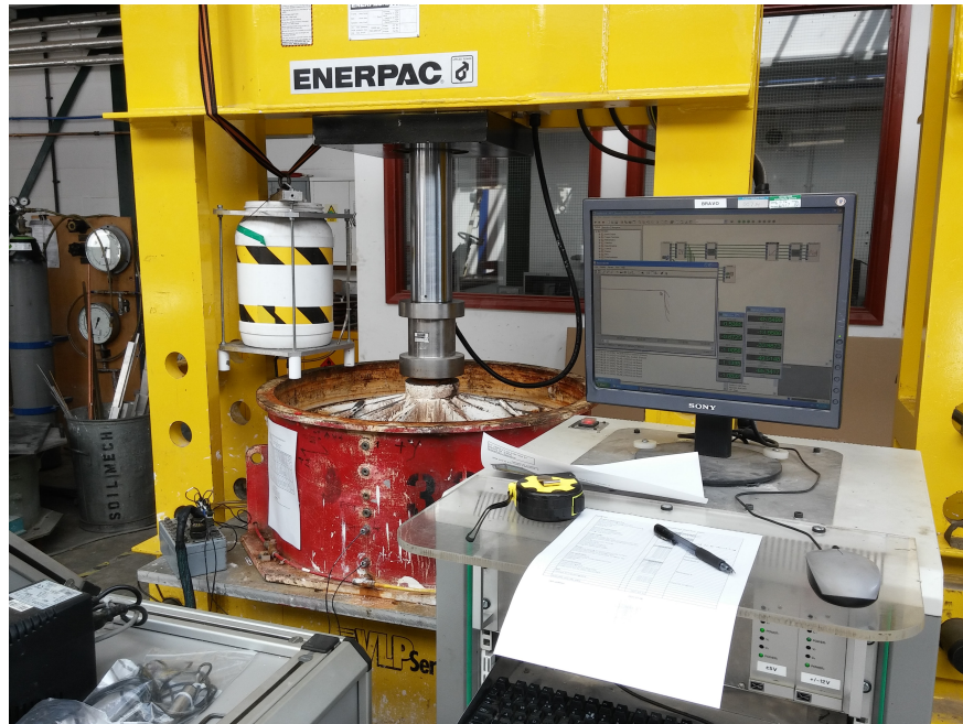
Fig. 6. Photograph of clay layer compressed and monitored in hydraulic consolidometer
