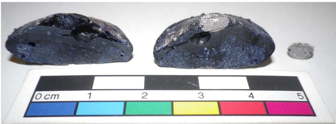
**Figure 31** The sectioned sample showing the cobalt-blue glass and the metallic bead. Unreacted silica can be seen in the glass part. Note that the sample has been inverted from its position in the conical carbon crucible, i.e. the metallic phase was at the bottom.
