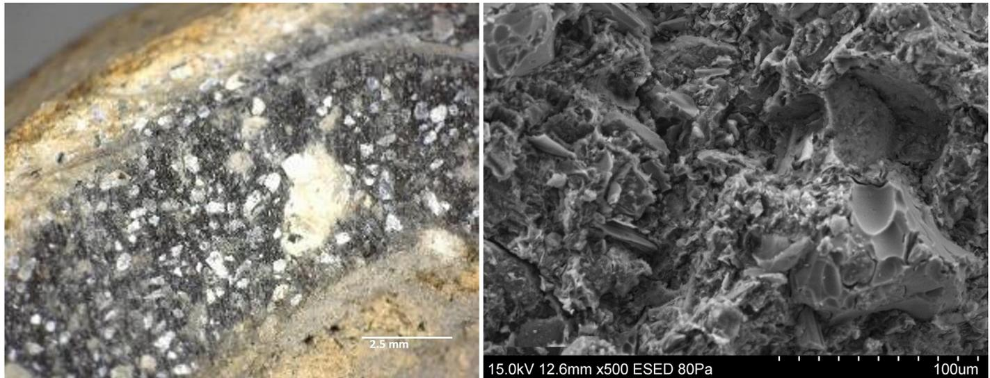
**Fig 12. Micro and macrostructural evidence of heat treatment in sample IN01.** A. Cross section showing the complete section with bright edges and a dark core. B. SEM image showing the microstructure without vitrification.
