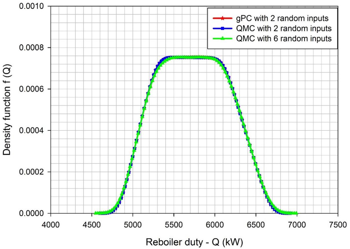
**Fig. 3.** Density distributions of the reboiler duty in the PG production process with six and two uniform random inputs (Example 1).
