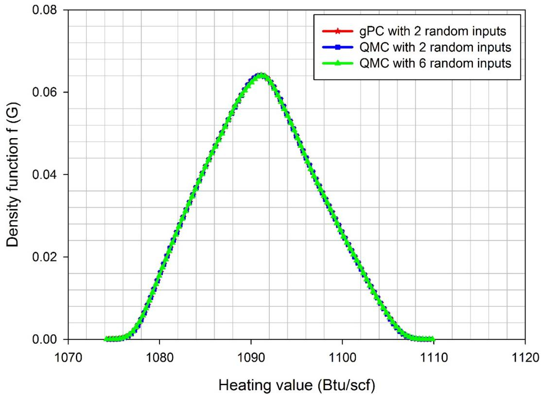
**Fig. 5.** Density distributions of the net heating value of sale gas in the lean dry gas production process with six and two uniform random inputs (Example 2).
