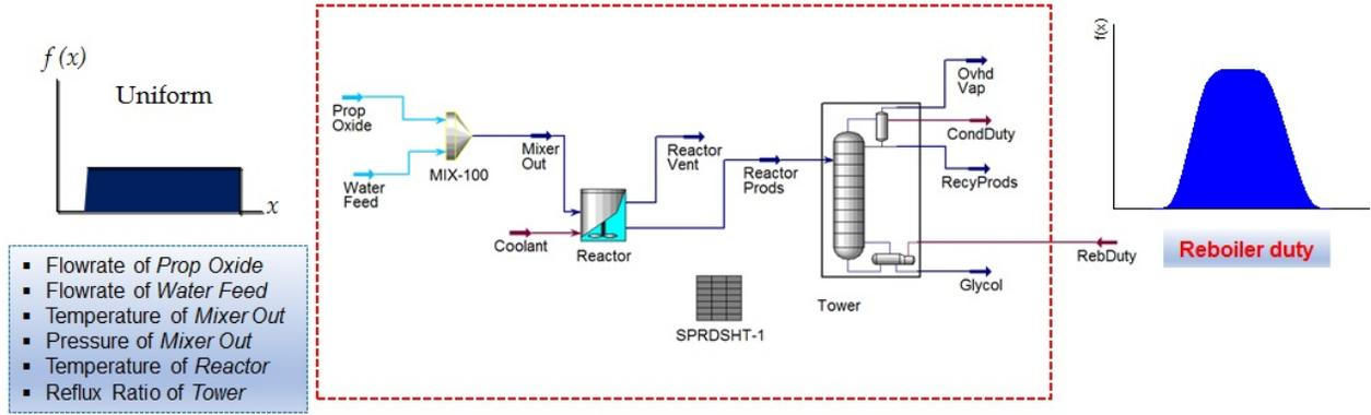
Fig. 2. Propylene glycol (PG) production process (Example 1).
