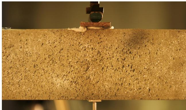
Figure 2. Example of field of view of DIC images showing speckle pattern applied to the concrete beam exterior
