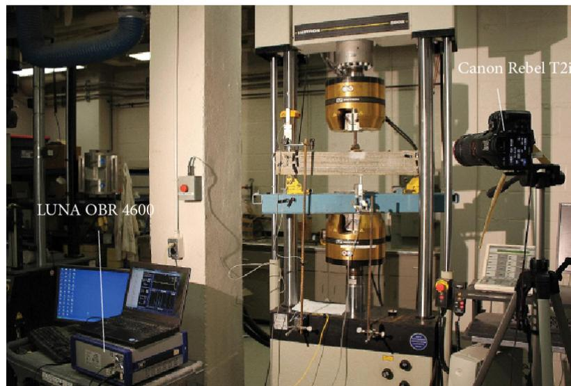
Figure 3. Test set-up including LUNA OBR 4600 and DIC camera orientation.
