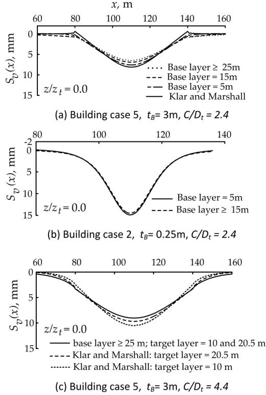
Figure 6: Effect of base layer thickness on soil-building interaction:  $V_{It} = 1.76\%$
