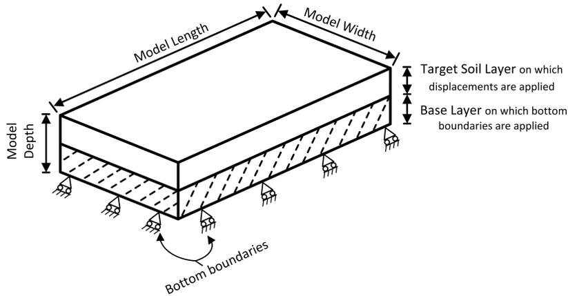
Figure 3: Mixed E–N model with base layer
