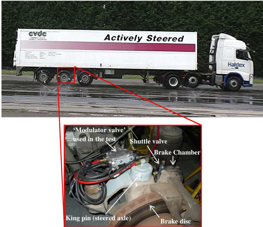
**Figure 7.** Test vehicle and high-speed modulator valve installed at wheel end
