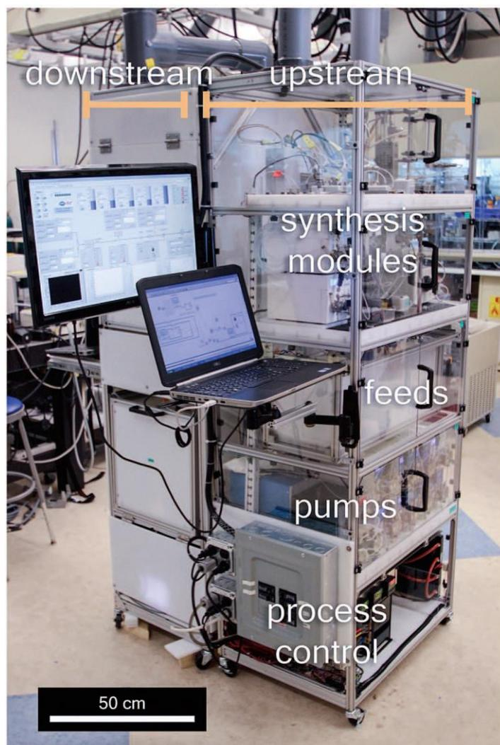
Figure 11. A compact synthesis unit capable of producing four APIs has been reported that uses common components for all target molecules. A control system switches individual unit operations into and out from the flow line to manage each synthesis. From [55]. Reprinted with permission from AAAS.
