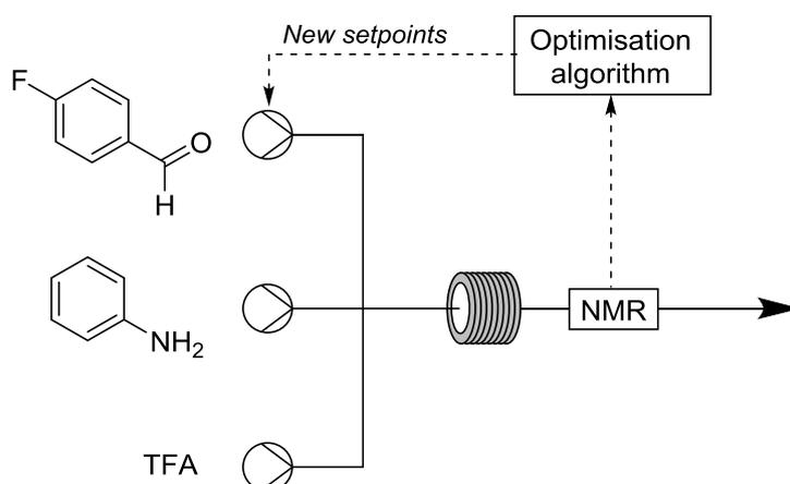
Figure 9. NMR was used to provide reaction performance feedback to drive the self-optimisation of an imine formation reaction. Reproduced from [44] – published by the Royal Society of Chemistry.
