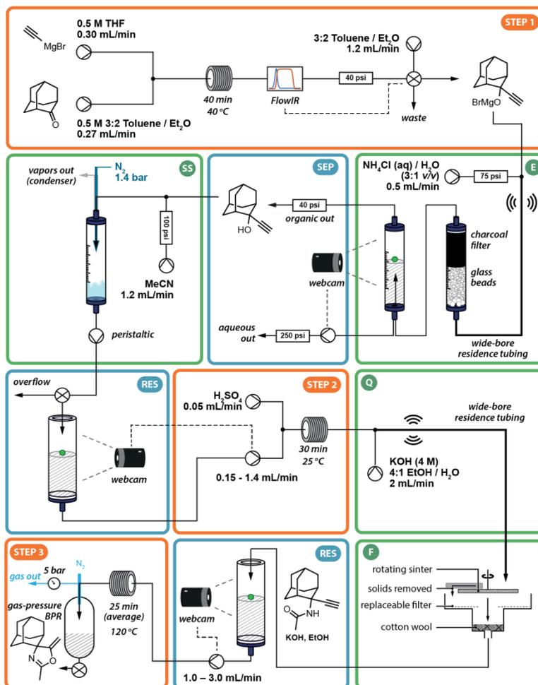
Figure 12. Three transformation steps were telescoped using commercially available laboratory equipment, incorporating a number of downstream processing steps. Custom Python scripts were used to automate the process.
