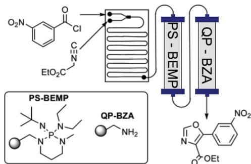
Figure 4. a) the level of technical integration for the synthesis of 4,5-disubstituted oxazoles was enabled through the use of a computer control system. Items outlined in red represent those with direct feedback and control by the computer; b) Example transformation carried out in a single process. Reprinted with permission from [14]. Copyright 2006 American Chemical Society.
