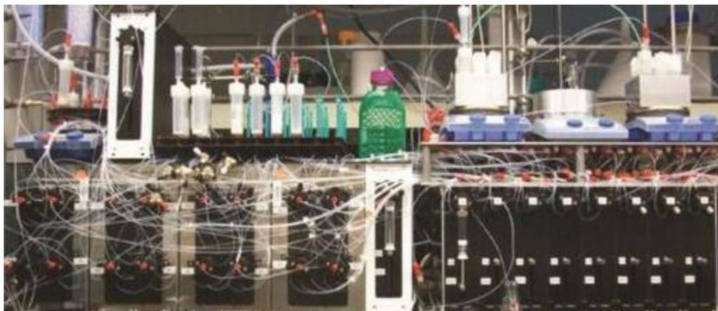
Figure 10. The system designed by Burke *et al.* consisted of a number of pumps, switching valves and reaction sections to iteratively perform deprotection, coupling and purification steps. From [53]. Reprinted with permission from AAAS.
