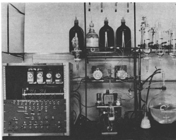
Figure 1. Apparatus used to automate solid-phase peptide synthesis in 1965. The “programmer” on the left was responsible for controlling reaction sequences. From [12]. Reprinted with permission from AAAS.
