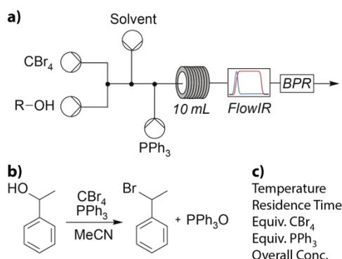
Figure 15. a) Equipment schematic for the five dimensional optimisation; b) reaction scheme; c) the five parameters manipulated by the control system during the optimisation process. Reproduced from [10].
