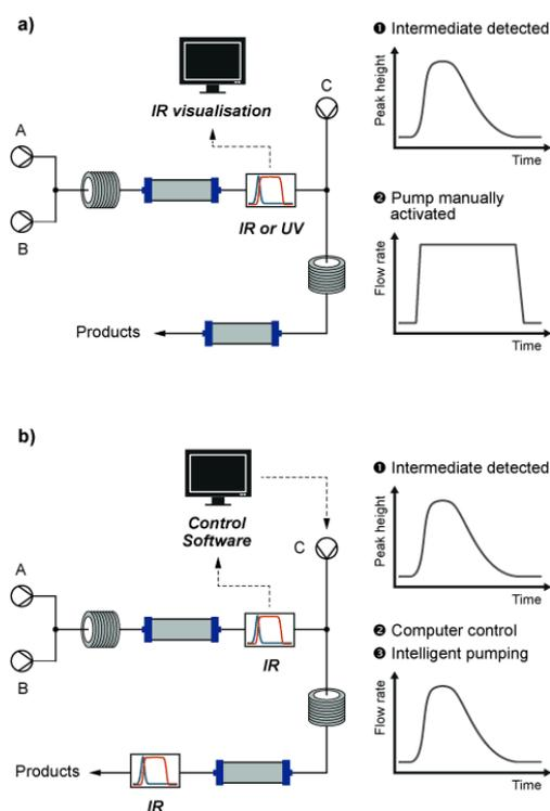
Figure 5. Feedback from an IR spectrometer was used to control downstream pump flowrates to precisely match stoichiometry. Reproduced with permission from John Wiley and Sons, reference [2].
