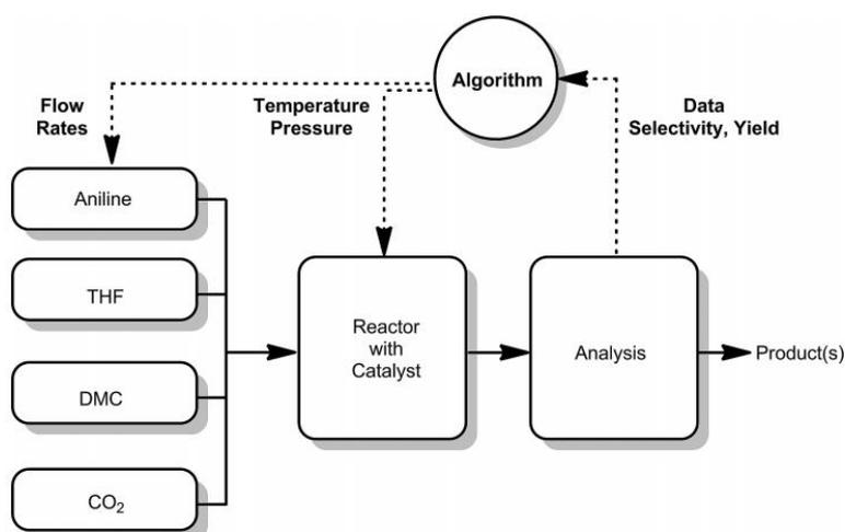
Figure 6. Schematic showing the feedback information flow used to optimise for each of the products and byproducts observed when aniline and dimethyl carbonate were reacted the presence of THF over an alumina catalyst. Figure reproduced with permission from John Wiley and Sons, reference [25].
