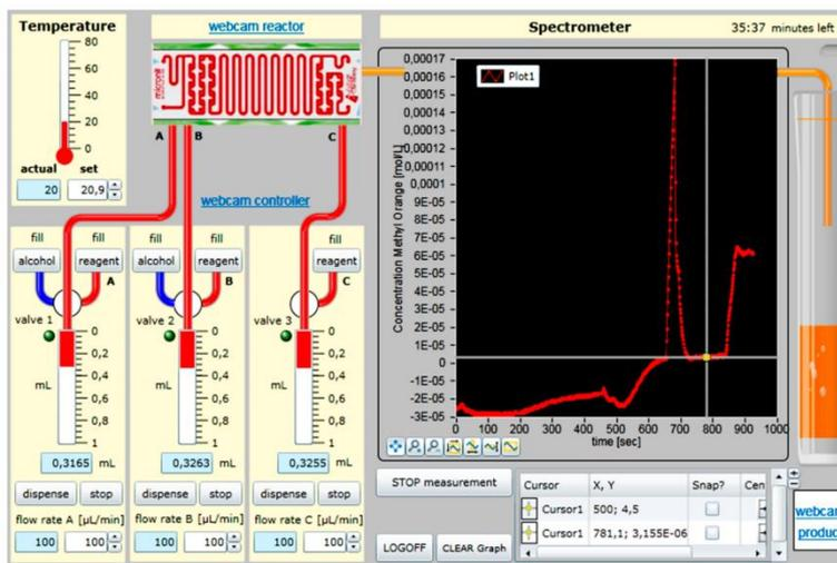
Figure 13. The web interface shown to students, enabling them to control and monitor the reaction remotely. Reprinted with permission from [63]. Copyright 2013 American Chemical Society.
