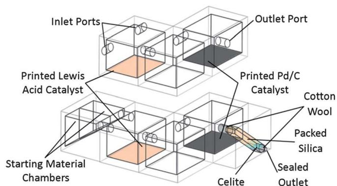
Figure 16. The 3D printed vessels included a number of reaction chambers, including those that incorporated catalysts printed onto surfaces. Reproduced from [75] - published by The Royal Society of Chemistry.
