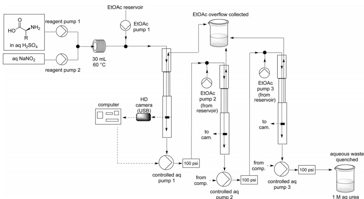
Figure 8. Multiple extraction columns in series have been used for more complex extraction situations, especially when reaction components are soluble in both the aqueous and organic phases. Reprinted with permission from [32]. Copyright 2012 American Chemical Society.
