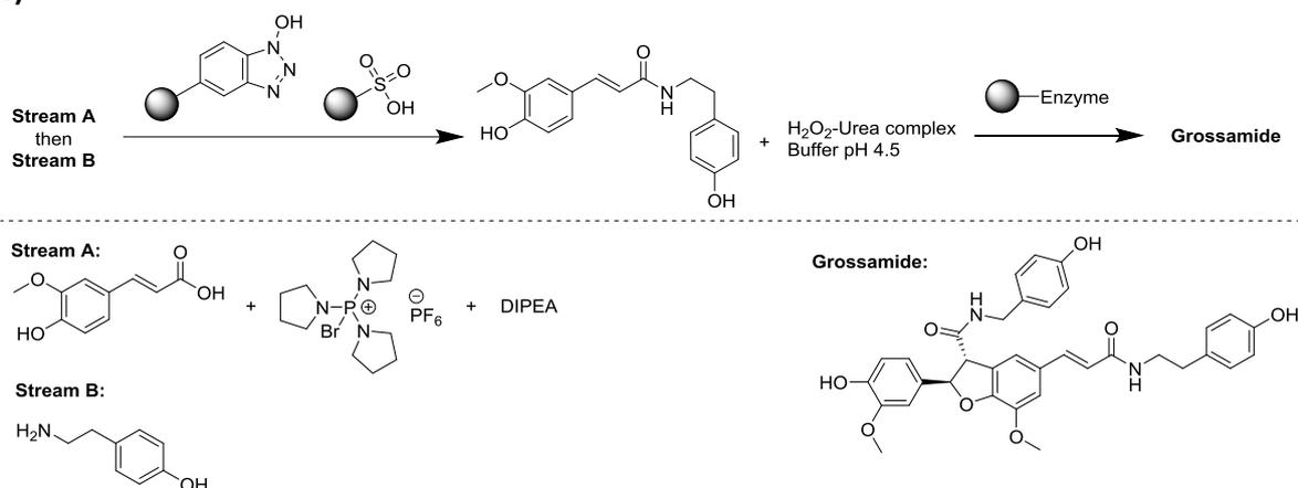
Figure 2. a) the synthesis of grossamide was enabled through the use of an automated control system. Reproduced with permission, reference [13]; b) the synthetic pathway selected to prepare Grossamide.
