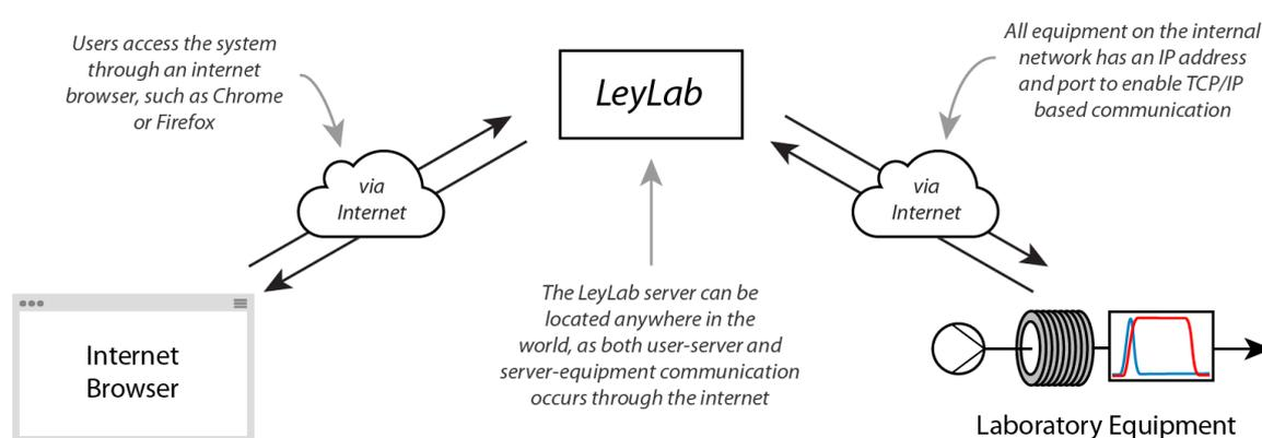
Figure 14. Our reported control system is fully cloud-based, with all communication occurring through TCP/IP. Users access the system through an internet browser. Reproduced from [10].
