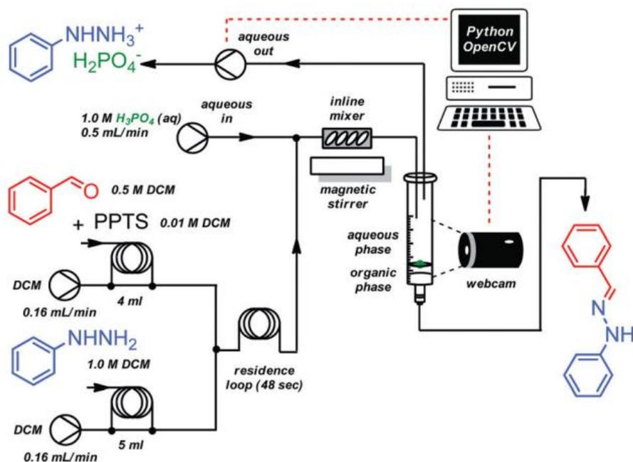
Figure 7. Schematic of an automated, inline liquid-liquid separator system powered with open-source technologies.[31] Reproduced by permission of The Royal Society of Chemistry.
