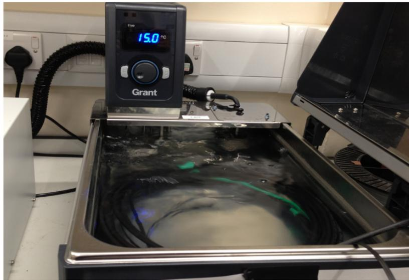
Fig. 3.27 Temperature calibration bench of a water bath
