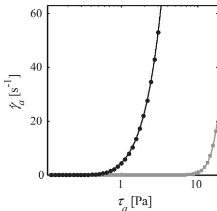
**Fig. 6.** Apparent shear rate-shear stress data for the (●) 0.1 and (■) 0.2 wt% Carbopol 940 solutions obtained using conventional rheometry. The symbols show the experimentally acquired data and the solid lines show the regression data. Regression was performed over the shear rate range of the NMR experiments using Eq. (19).
