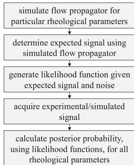
Fig. 2. Block diagram outlining the key stages in the proposed Bayesian NMR approach.
