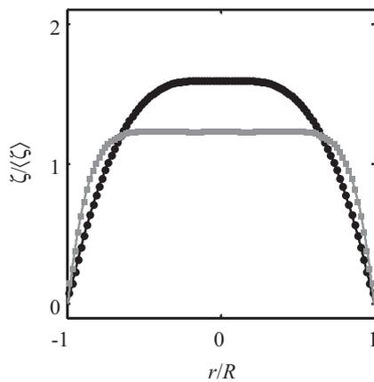
**Fig. 14.** Displacement profiles, generated from radially-averaged 2D velocity image data, shown for the (●) 0.1 and (■) 0.2 wt% Carbopol 940 solutions, with fluid displacement and radial position represented as a fraction of the mean fluid displacement and pipe radius, respectively. The solid lines represent the radially-averaged 2D regression data, with the fitted data within the accuracy of the experimental data.
