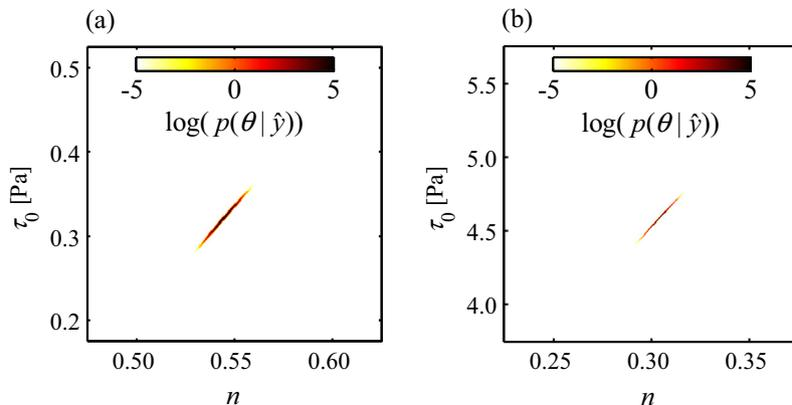
**Fig. 12.** 2D posterior probability distributions, plotted on a log scale, showing the probability of  $n$  and  $\tau_0$  given  $\hat{y}$  for the (a) 0.1 and (b) 0.2 wt% Carbopol 940 solutions. The SNR (at  $q = 0 \text{ m}^{-1}$ ) is >1000, with the 128 points in  $q$ -space sampled using the experimental procedure outlined in Section 3.2.2.
