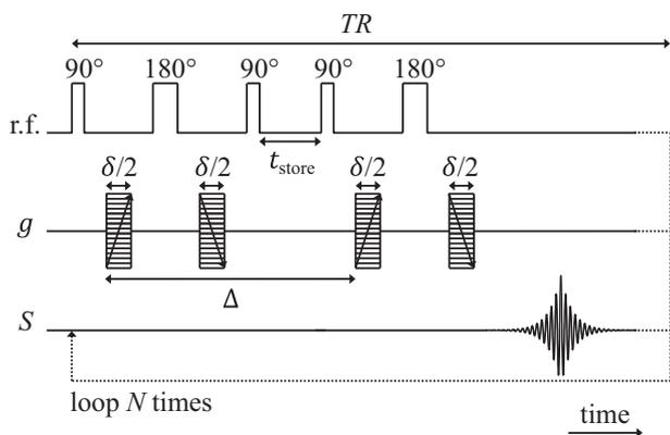
Fig. 5. Schematic of the 13-interval APGSTE sequence used for the acquisition of the volume-averaged flow propagator and data for Bayesian analysis.
