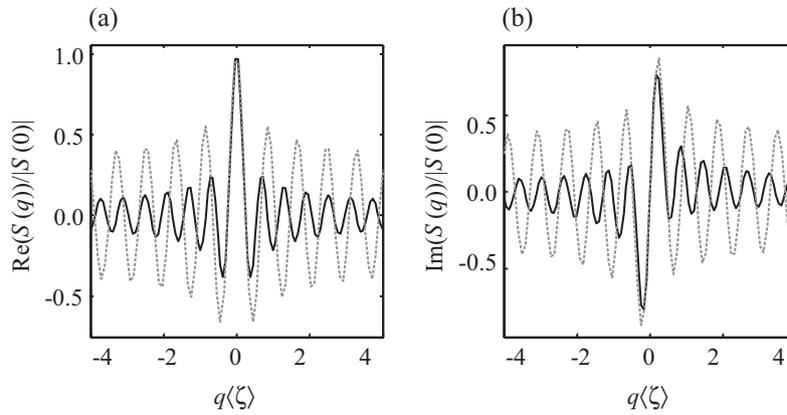
**Fig. 10.** Experimental results showing the evolution of the normalised (a) real and (b) imaginary components of the experimentally acquired  $S(q)$ , plotted across a  $q$ -space range of  $\pm 4\langle\zeta\rangle^{-1} \text{ m}^{-1}$  for the (—) 0.1 and (---) 0.2 wt% Carbopol 940 solutions; SNR > 1000.
