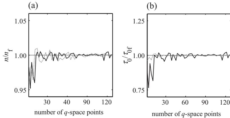
**Fig. 13.** Plots to demonstrate the relationship between the number of points sampled in  $q$ -space and (a)  $n$  and (b)  $\tau_0$  values obtained for the (—) 0.1 and (---) 0.2 wt% Carbopol 940 solutions. For clarity, the  $n$  and  $\tau_0$  values are represented as a fraction of those parameters obtained using 128 sampled  $q$ -space data points ( $n_f$  and  $\tau_{0f}$ , respectively). The horizontal line (· · ·) represents the ideal result.
