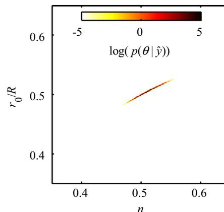
**Fig. 7.** A 2D posterior probability distribution, plotted on a log scale, showing the probability of  $n$  and  $r_0/R$  given the experimental observations  $\hat{y}$  obtained using simulated data. The data were generated with 128 sampled  $q$ -space data points and SNR of 100 for a ground truth of  $n = 0.5$  and  $r_0/R = 0.5$ .
