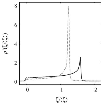
**Fig. 11.** Experimentally acquired flow propagators for the (—) 0.1 and (---) 0.2 wt% Carbopol 940 solutions. Displacement is represented as a fraction of mean fluid displacement.
