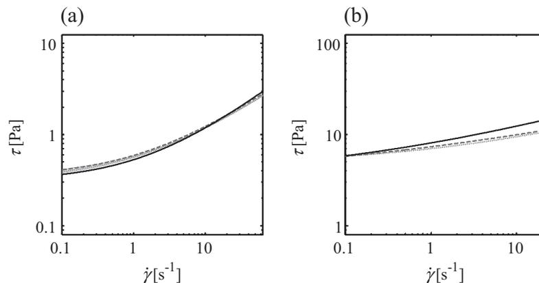
**Fig. 15.** Flow curves for the (a) 0.1 and (b) 0.2 wt% Carbopol 940 solutions obtained using (—) conventional rheometry, (---) MR flow imaging, and (· · ·) Bayesian NMR, plotted across the shear rate ranges of the NMR experiments. The width of the line for the Bayesian NMR results represent the 95% confidence bands obtained from the 2D posterior probability distributions shown in Fig. 12.
