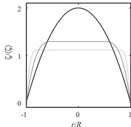
**Fig. 1.** Displacement profiles generated using Eq. (4) for three example fluids; with (—)  $n = 1.0$  and  $r_0/R = 0.0$ , (---)  $n = 0.5$  and  $r_0/R = 0.5$ , and (····)  $n = 0.5$  and  $r_0/R = 0.8$ . Fluid displacement and radial position are represented as a fraction of the mean fluid displacement and pipe radius, respectively.
