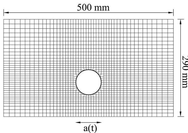
Figure 6. Mesh used in the 2D numerical analyses (model scale).
