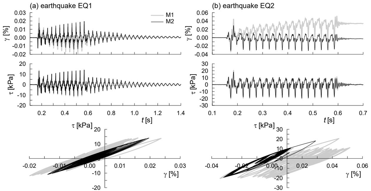
Figure 14. Test T4, free-field vertical,  $z = 0.182$  m. Shear strain and shear stress time histories and  $\tau$ - $\gamma$  cycles during earthquake (a) EQ1 and (b) EQ2.
