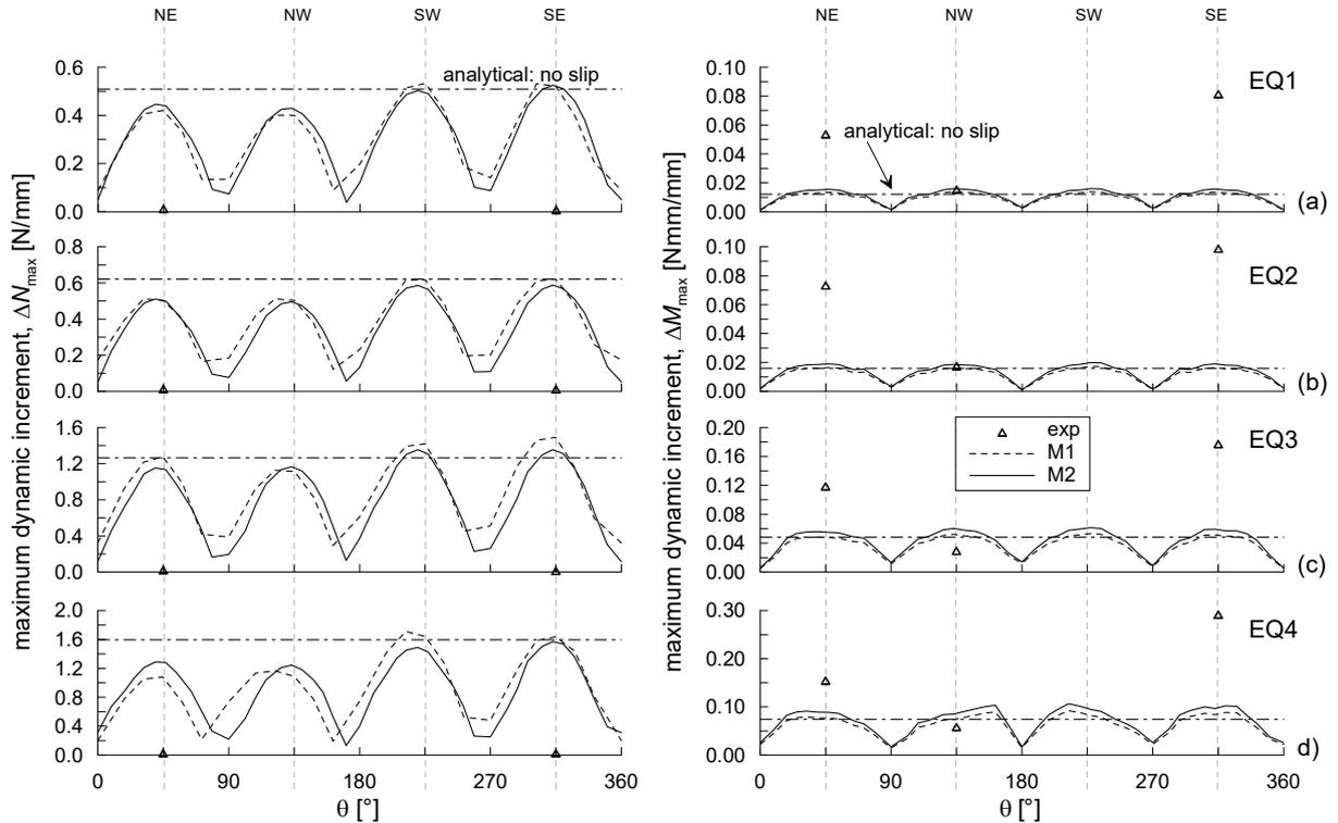
Figure 13. Test T4. Dynamic increment of bending moments and hoop forces in the lining during earthquakes: (a) EQ1, (b) EQ2, (c) EQ3 and (d) EQ4. Comparison between experimental data, numerical results and analytical solutions.
