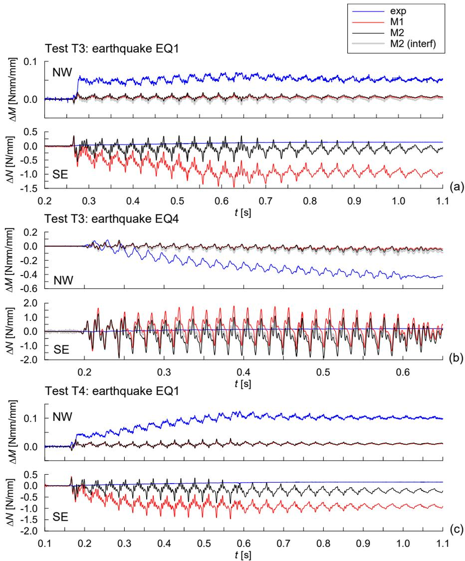
Figure 11. Dynamic increment of bending moment (NW) and hoop force (SE) in the lining during earthquakes: (a) EQ1 and (b) EQ4 of test T3 and (c) EQ1 of test T4. Comparison between experimental data and numerical results.
