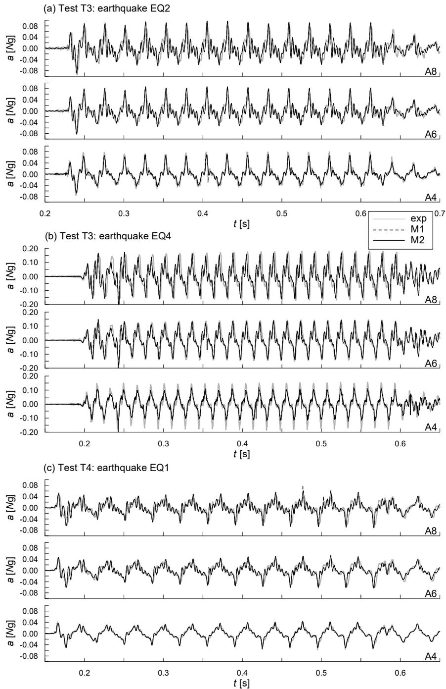
Figure 8. Accelerations along the tunnel vertical (A4, A6, A8) during earthquakes: (a) EQ2 and (b) EQ4 of test T3 and (c) EQ1 of test T4. Comparison between experimental data and numerical results.
