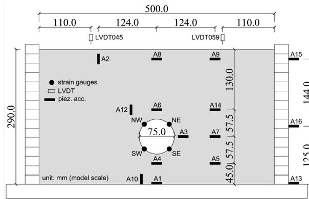
Figure 1. Test T3 and T4: transducers layout
