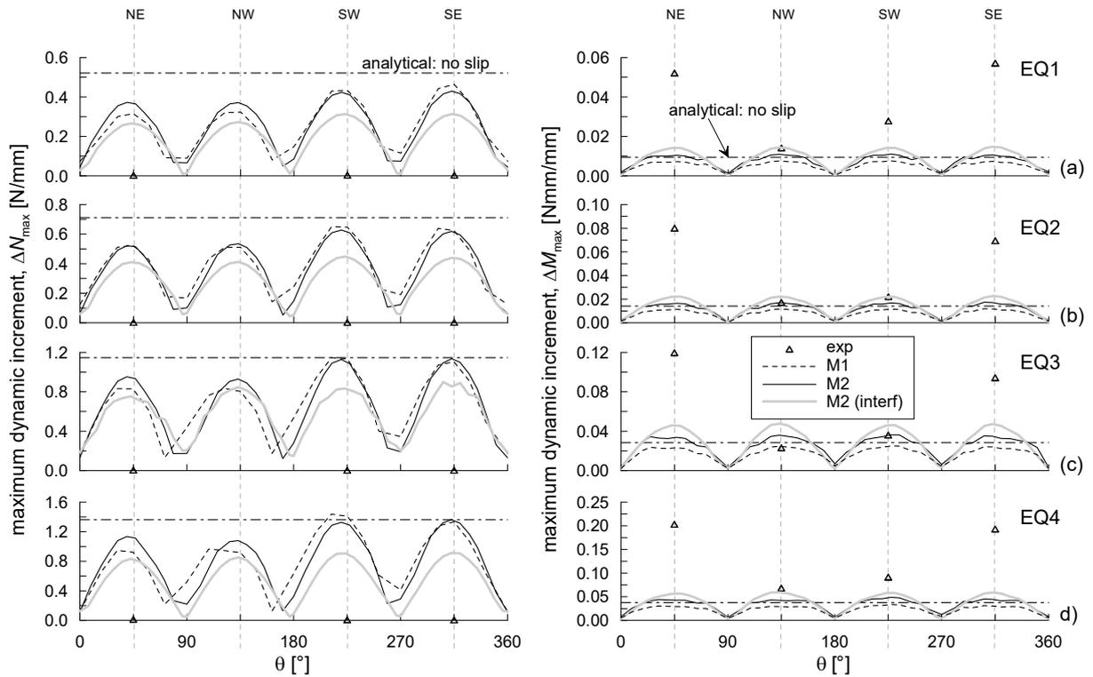
Figure 12. Test T3. Maximum dynamic increment of bending moments and hoop forces in the lining during earthquakes: (a) EQ1, (b) EQ2, (c) EQ3 and (d) EQ4. Comparison between experimental data, numerical results and analytical solutions.
