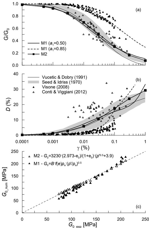
Figure 3. Model M1 and M2. Calibration of model constants from laboratory and centrifuge data: (a) shear modulus degradation curve, (b) damping ratio and (c) small strain shear modulus
