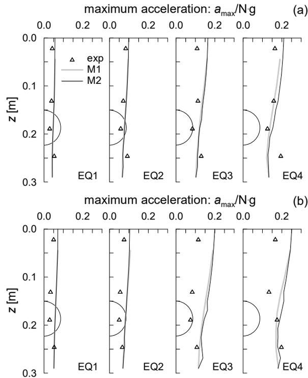
Figure 9. Free-field vertical, distribution of maximum accelerations during the four earthquakes applied: (a) test T3 and (b) test T4). Comparison between experimental data and numerical results.
