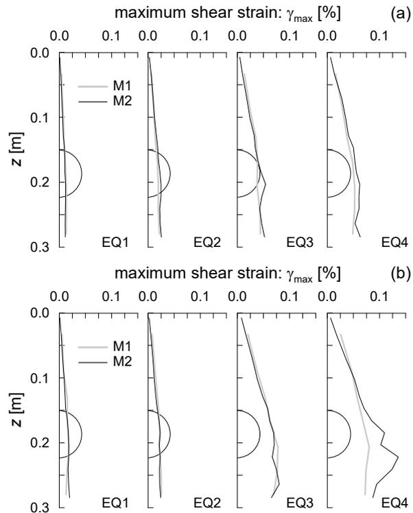
Figure 10. Free-field vertical, distribution of maximum shear strain during the four earthquakes applied: (a) test T3 and (b) test T4).
