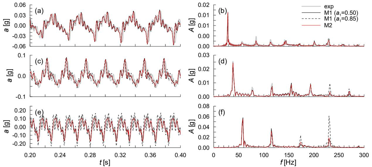
Figure 5. Test T4: 1D wave propagation analyses for EQ2 (accelerometer A9: a, b), EQ4 (accelerometer A14: c, d) and EQ1 (accelerometer A9: e, f). Comparison between experimental data and numerical results.
