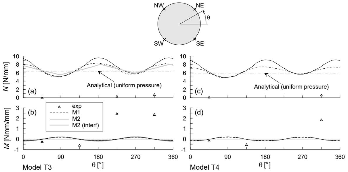
Figure 7. Distribution of bending moments and hoop forces in the lining after the swing up stage for: (a, b) model T3 and (c, d) model T4.
