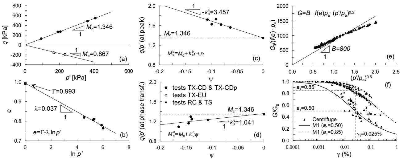
Figure 2. Model M1: calibration of model constants from experimental data.
