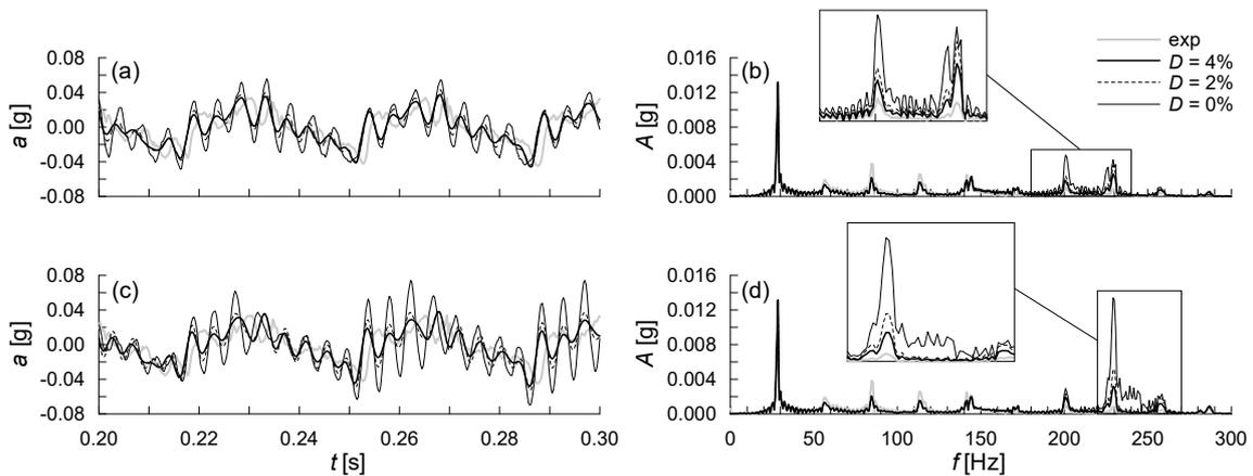
Figure 4. Test T4, earthquake EQ1 (accelerometer A9): 1D wave propagation analyses with soil model M1: (a,b)  $a_1 = 0.50$  and (c,d)  $a_1 = 0.85$ . Comparison between experimental data and numerical results obtained with different values of the Rayleigh damping.
