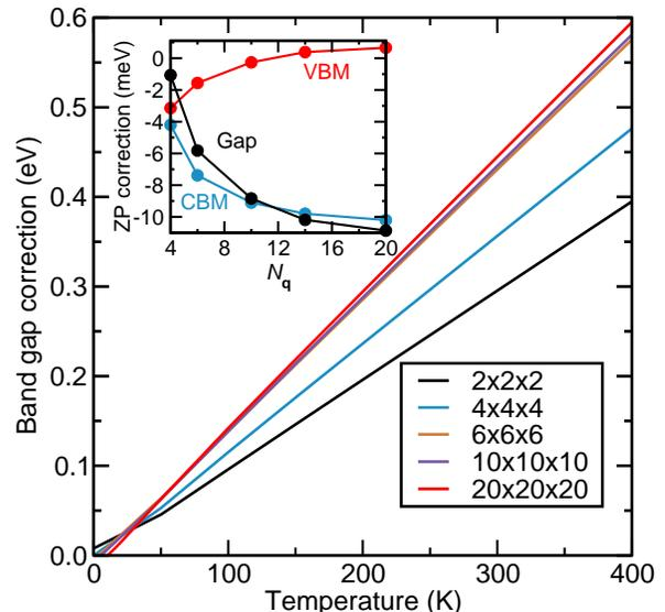
FIG. 1. Temperature dependence of the band gap of MAPbI<sub>3</sub> evaluated using the AHC approach with different BZ grids of sizes  $N_{\mathbf{q}}^3$ . The inset shows the convergence of the VBM, CBM and band gap ZP corrections at the  $\mathbf{R}$ -point as a function of the vibrational BZ grid linear size.
