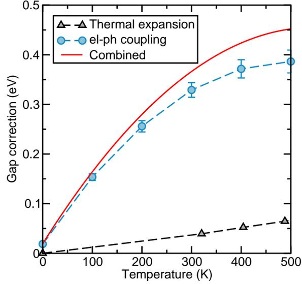
FIG. S7. Temperature dependence of the band gap of MAPbI<sub>3</sub> evaluated using thermal expansion only (black triangles), electron-phonon coupling only with MC and SOC on a  $3 \times 3 \times 3$  supercell (blue circles), and both (red dashed-dotted line). The statistical error bars are included in all MC data points, although they are not visible in some as their size is smaller than the symbol size.
