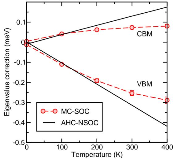
FIG. S6. Temperature dependence of the individual eigenvalues at the valence (lower lines) and conduction (upper lines) band at the **R**-point of the BZ. The calculations have been performed using the same numerical parameters as those in Fig. 3 of the main manuscript, but without the inclusion of thermal expansion.
