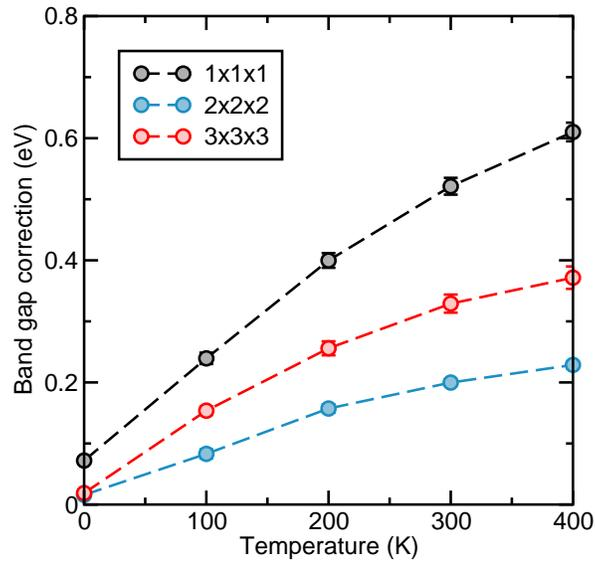
FIG. S3. Temperature dependence of the band gap of MAPbI<sub>3</sub> evaluated using supercells of sizes  $1 \times 1 \times 1$  (black circles),  $2 \times 2 \times 2$  (blue circles), and  $3 \times 3 \times 3$  (red circles). The statistical error bars are included in all data points, although they are not visible in some as their size is smaller than the symbol size.
