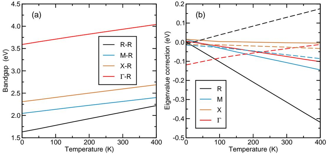
FIG. S5. (a) Temperature dependence of band gaps of MAPbI<sub>3</sub> from the VBM at the **R** point to the conduction band of several high-symmetry points in the BZ. (b) Temperature dependence of the individual eigenvalues at the valence (solid lines) and conduction (dashed lines) band at several high-symmetry points of the BZ. All calculations have been performed using the PBE functional and the AHC theory. The SOC and thermal expansion are not included.
