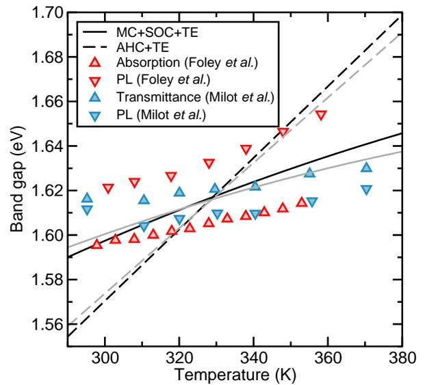
FIG. 3. Temperature dependence of the band gap of  $\text{MAPbI}_3$  from Foley *et al.* [15] and from Milot *et al.* [16] using various techniques (red and blue triangles respectively), compared to the theoretical prediction using the MC approach (black solid line) and the AHC theory (dashed black line). Both theoretical lines include the effects of thermal expansion, but only the MC line includes SOC. The results neglecting thermal expansion are shown with grey lines.
