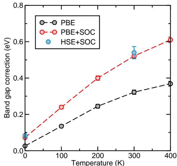
FIG. S2. Temperature dependence of the band gap of MAPbI<sub>3</sub> evaluated using PBE (black circles), PBE+SOC (red circles), and HSE+SOC (blue circles), and the MC method. Only the electron-phonon coupling constants for  $\Gamma$ -point phonons are included. The statistical error bars are included in all data points, although they are not visible in some as their size is smaller than the symbol size.
