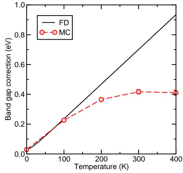
FIG. S8. Temperature dependence of the band gap of CsPbI<sub>3</sub> evaluated using the FD and MC methods. The calculations have been performed using the PBE functional, with a  $2 \times 2 \times 2$  BZ grid, and without including SOC. Statistical error bars are included in the MC data points, but they are not visible for some data points as they are smaller than the symbols.
