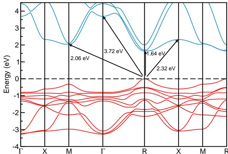
FIG. S4. Static lattice band structure of MAPbI<sub>3</sub> calculated using the PBE functional without including SOC. The dashed line indicates the position of the Fermi level.
