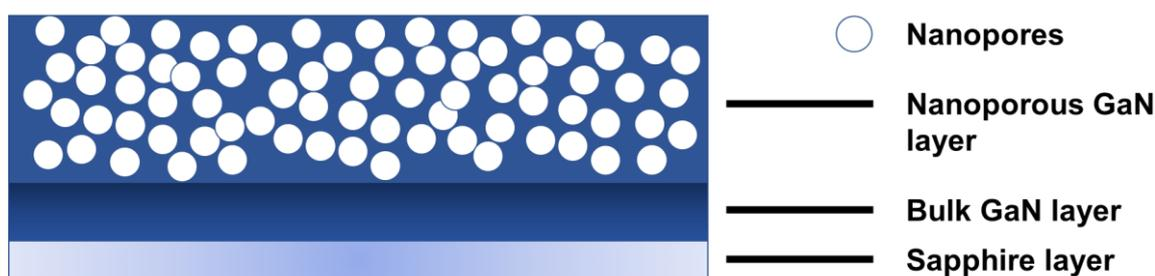
Figure 4-3 Illustration of the cross-section of nanoporous GaN samples utilised in this research. GaN samples consist of a nanoporous GaN layer, a bulk GaN layer and a sapphire layer.
