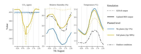
Figure 7. Effect of the plant module on temperature, relative humidity and CO<sub>2</sub> concentration for one day in August. The line type refers to the simulation level: dotted - GES-II output at the end of the timestep, solid - updated BES output after input from GES-II. The planted level indicates the outputs for the two scenarios: "No plants" ( $A_p = 1\%$  of floor area) and "Full plants" ( $A_p = 98\%$  of floor area).
