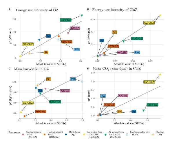
Figure 9. Comparing SRC coefficients (-) and Morris method elementary effects ( $\mu$ \*) for four annual model outcomes: (A) energy use intensity of the greenhouse (kWh/m<sup>2</sup>/year), (B) energy use intensity of the ClaZ (kWh/m<sup>2</sup>/year), (C) total Dry Matter grown over 1 year per unit of cultivated area (kgDM/m<sup>2</sup>/year), and (D) mean CO<sub>2</sub> in ClaZ on occupied days between 8pm and 6am (ppm).
