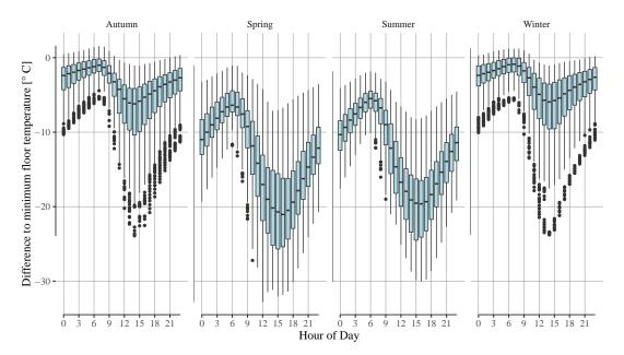
Figure 6. The difference of floor temperature with and without a large rooftop window (area of  $0.85A_{GZ}$ ), separated by seasons.
