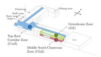
Figure 3. Representation of the school building model, with the three zones of interest: (1) the Greenhouse Zone (GZ), (2) the top floor Corridor Zone (CorZ), and (3) the south facing Classroom Zone on the middle floor (ClaZ).
