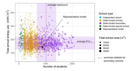
**Figure 2.** Energy Use Intensity (thermal and electrical) of the 3309 schools in Central London, plotted against headcount of students. Data from combined DEC certificates and National Statistics for Schools merged by postcode. The black point shows where the representative model situates itself. The mean (dotted line) and standard deviation (purple band) for secondary schools are represented with purple lines.
