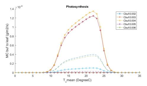
Figure A1. Flow of CH<sub>2</sub>0 from the buffer to the leaf  $MC_{buf \rightarrow leaf}$  (straight line), and from the leaf to the air  $MC_{leaf \rightarrow air}$  (dotted line, maintenance respiration).
