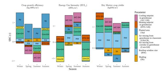
Figure 10. SRC calculated for four seasonal subsets for three model outcomes: (A) crop growth efficiency (g fresh weight (FW)/kWh), (B) total EUI of ClaZ and GZ, and (C) accumulated Dry Matter over a year per unit of cultivated area.
