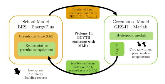
**Figure 5.** Co-simulation setup between the Greenhouse Zone (GZ) of the BES model in EnergyPlus and GES-II in Matlab. The curved arrows symbolise the exchanged data between the two models at each timestep. The straight black arrows indicate the stored data in each model.
