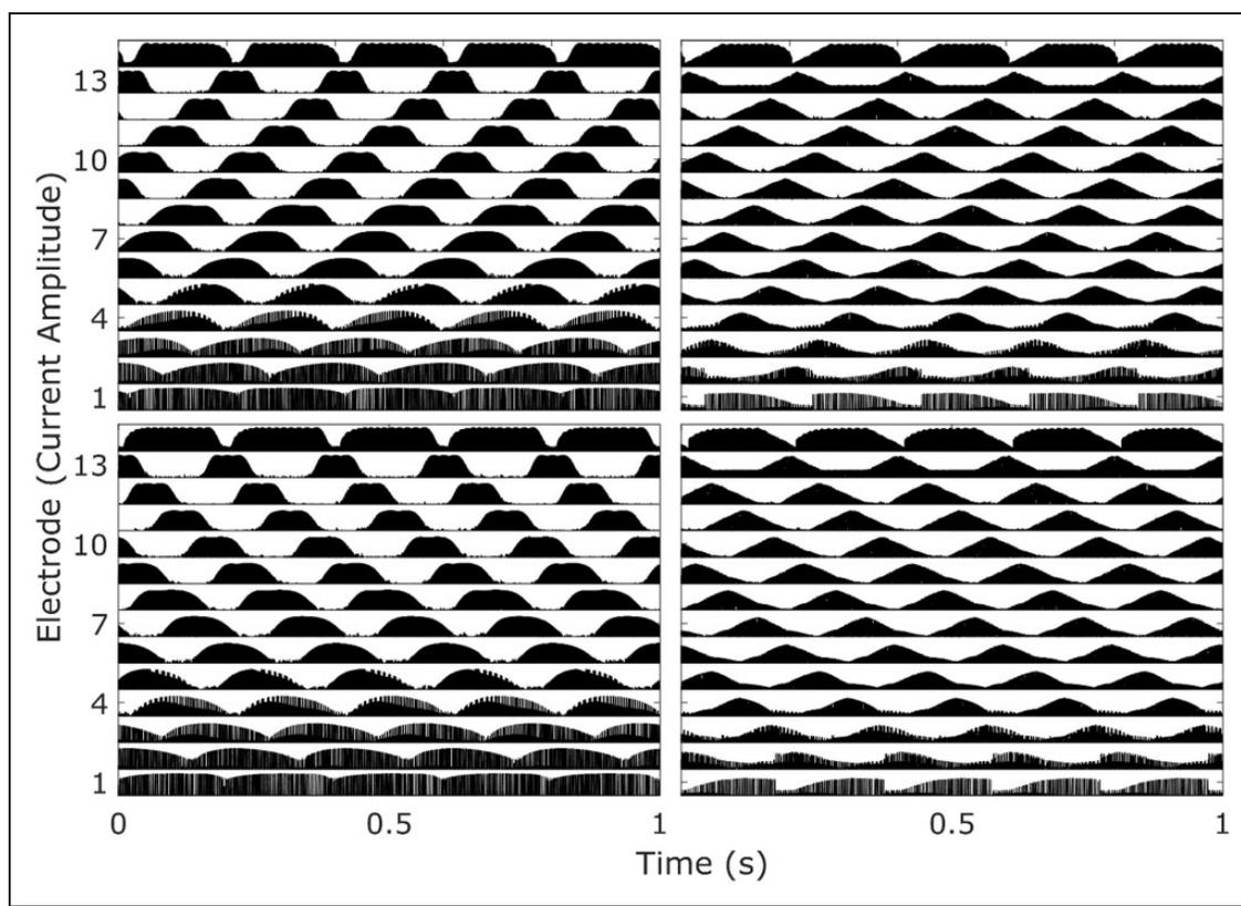
**Figure 4.** Electrodegram Plots of Density = 5 STRIPES Stimuli When Processed Using AB24's HiRes (Left Panel) and Optima (Right Panel) Programs. The top row shows UP STRIPES, and the bottom row shows DOWN STRIPES.
