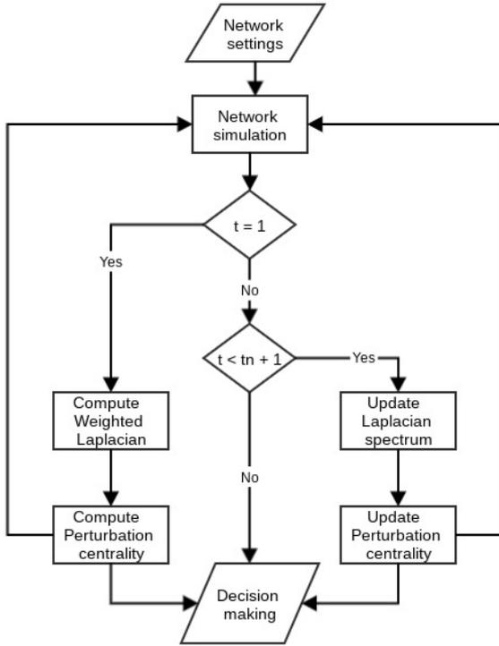
Fig. 1. Flowchart of any decision making using temporal perturbation centrality
