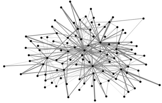
Fig. 2. Backbone for the UK communication network. Links are weighted by the average data traffic measured for 1 typical weekday. Geographical information is withheld to preserve anonymity.
