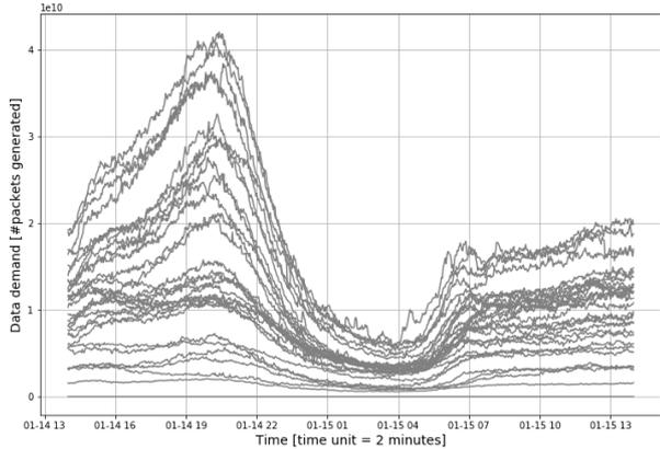
Fig. 4. Time series of 1 day of data traffic over the backbone network nodes
