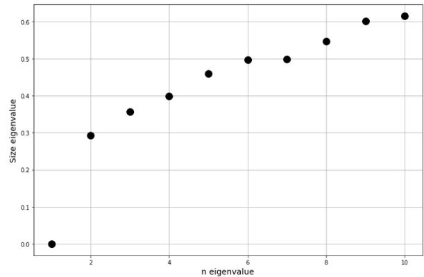
Fig. 3. First 10 eigenvalues of the unweighted, normalised Laplacian matrix of the UK backbone network
