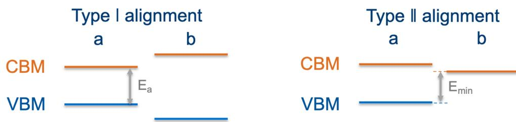
**Figure 5.21** Schematic diagram showing Type I and Type II band alignment.
