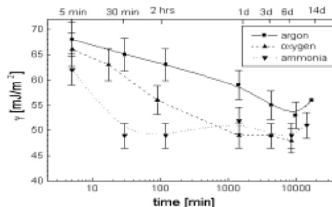
FIGURE 2. Ageing of surface free energy of PC after treatment in Ar, NH<sub>3</sub> and O<sub>2</sub> plasmas. The treatment conditions were P = 100 W, U<sub>bias</sub> = -25 V, Q = 52 sccm, p = 36.5 Pa. and treatment time t = 10 min. The bars in the graph correspond to standard deviation.
