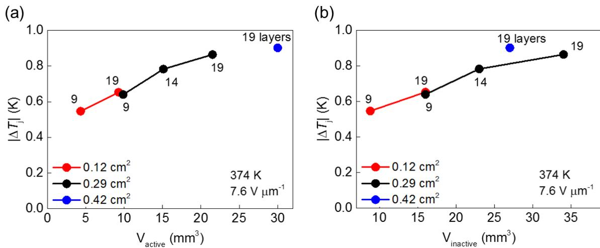
**Fig. S3. Dependence of measured temperature change on MLC geometry.** Variation of  $|\Delta T_j|$  with (a) active volume and (b) inactive volume, for an active area per layer of 0.12, 0.29 and 0.42  $\text{cm}^2$ .
