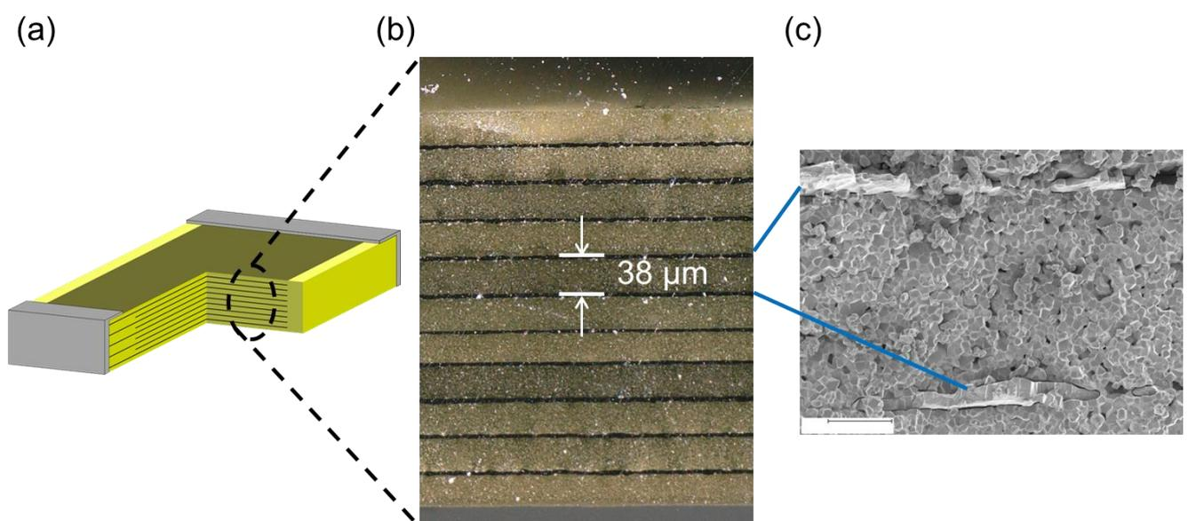
**Fig. S1. MLC structure.** (a) Schematic and (b,c) cross-sectional images obtained by (b) optical microscopy and (c) scanning electron microscopy.
