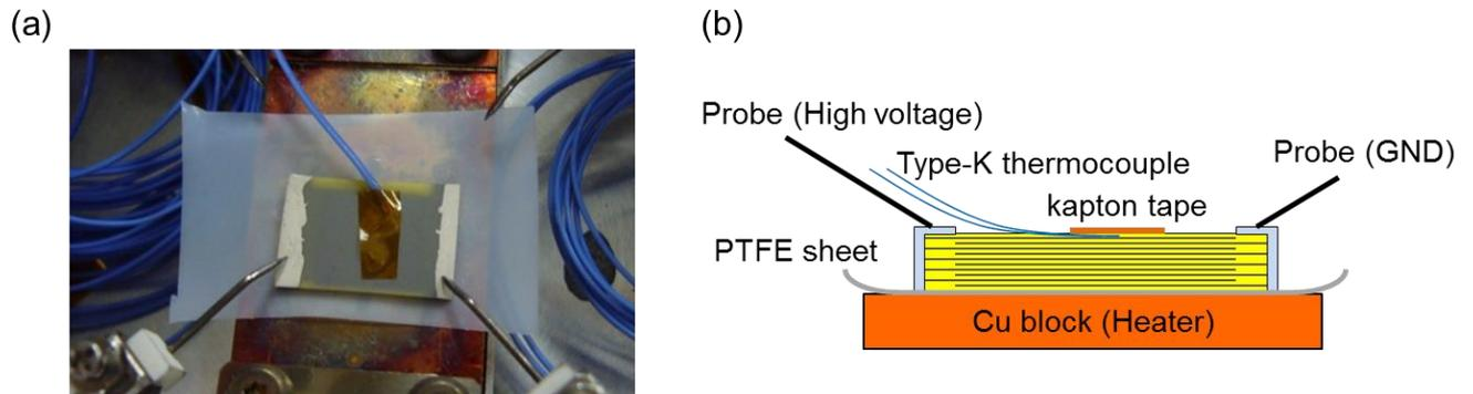
**Fig. S2. Measurement setup with the thermocouple.** (a) Photograph. (b) Schematic.
