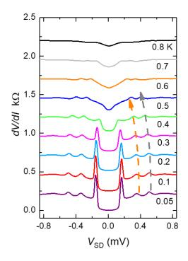
Figure 1. Multiple Andreev reflections and subharmonic gap structures in superconducting  $In_{0.75}Ga_{0.25}As$  two-dimensional electron gas: Temperature dependence induced superconductivity in 2DEG as a function of source-drain voltage  $V_{SD}$ . The pronounced SGS peaks due to multiple Andreev reflections in dV/dI ( $V_{SD}$ ) shift towards zero voltage bias when the base temperature is increased. The grey and orange dashed lines indicate the temperature evolution of the SGS.
