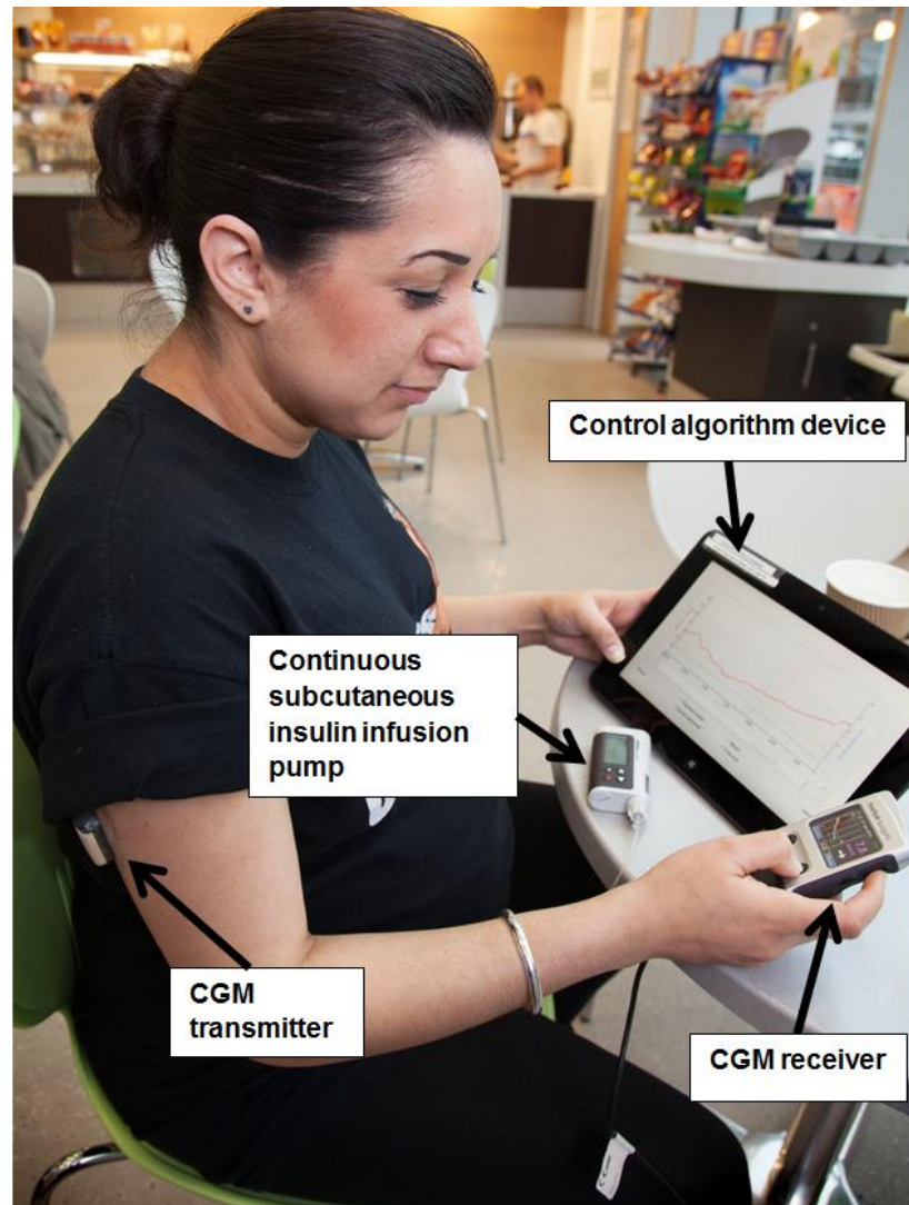
Figure 2.1: Participant wearing the closed-loop system
