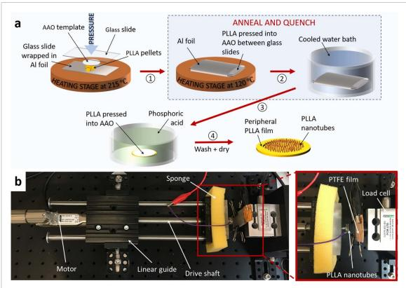
**Figure 1.** (a) Fabrication of PLLA NTs using melt press template wetting. (b) Linear motor setup for testing triboelectric devices. The sponge is used to prevent decreased contact area between the surfaces due to imperfections in the mounting angle of the samples. This is achieved by increasing the compliance of the system.
