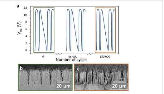
**Figure 4.** (a) Open circuit voltage of  $41 \pm 1\%$  crystalline PLLA NTs across several cycles. The same behaviour was seen in samples of lower crystallinity. (b) Cross section of NTs before use in and (c) after use in a TENG for 130 000 cycles.
