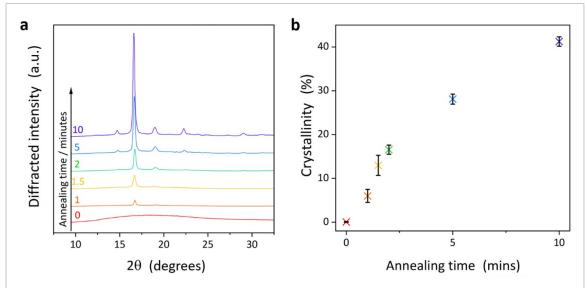
**Figure 2.** Crystallinity of PLLA NTs when annealed for different lengths of time. (a) XRD traces of a typical sample at each annealing time. (b) Calculated crystallinity using XRD spectra.
