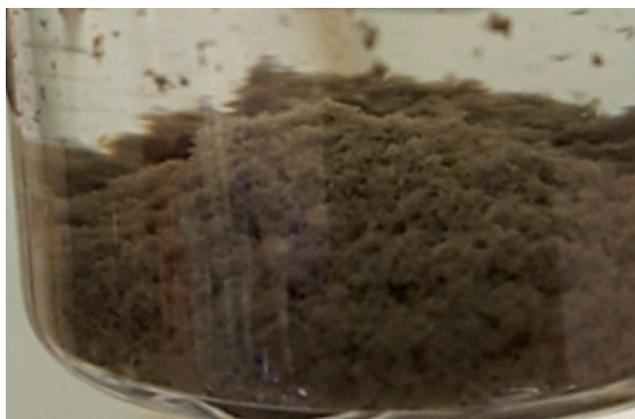
Figure 69: Photograph of silicon nanoparticle, carbon nanotube composite material in hexane.
