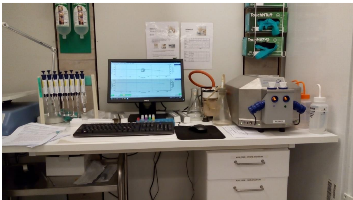
Figure 2.5. An Oxygraph in use measuring mitochondrial function in Hørsholm, Denmark during data collection for chapter 6 of this thesis.
