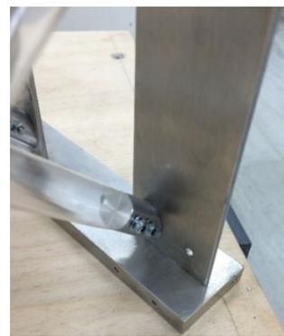
**Figure 3.2: Connection for partially hinged support and structural rocking, RA (a) and connection for fixed support and foundation rocking, RB (b)**
