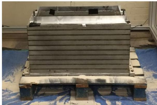
**Figure 4.4: Equivalent shear beam box**
