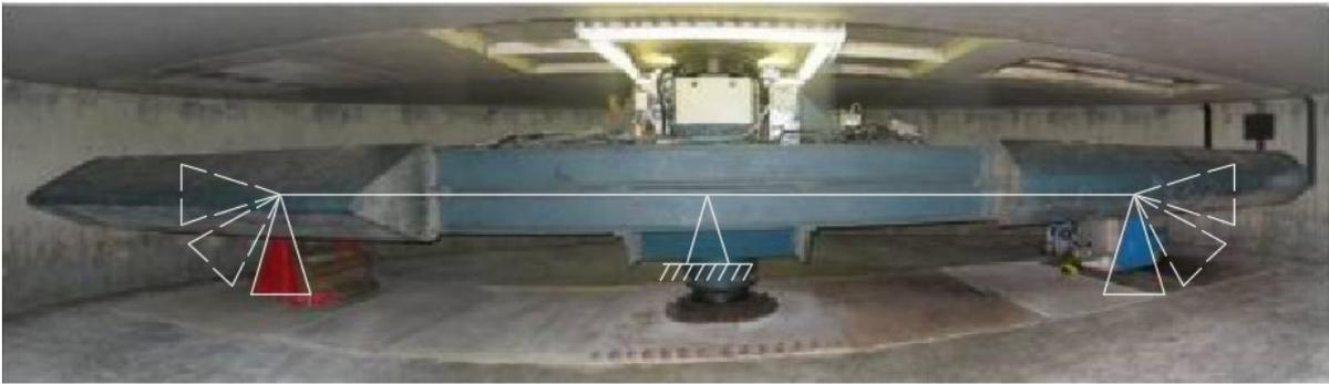
**Figure 4.1: The Turner beam centrifuge in Cambridge**
