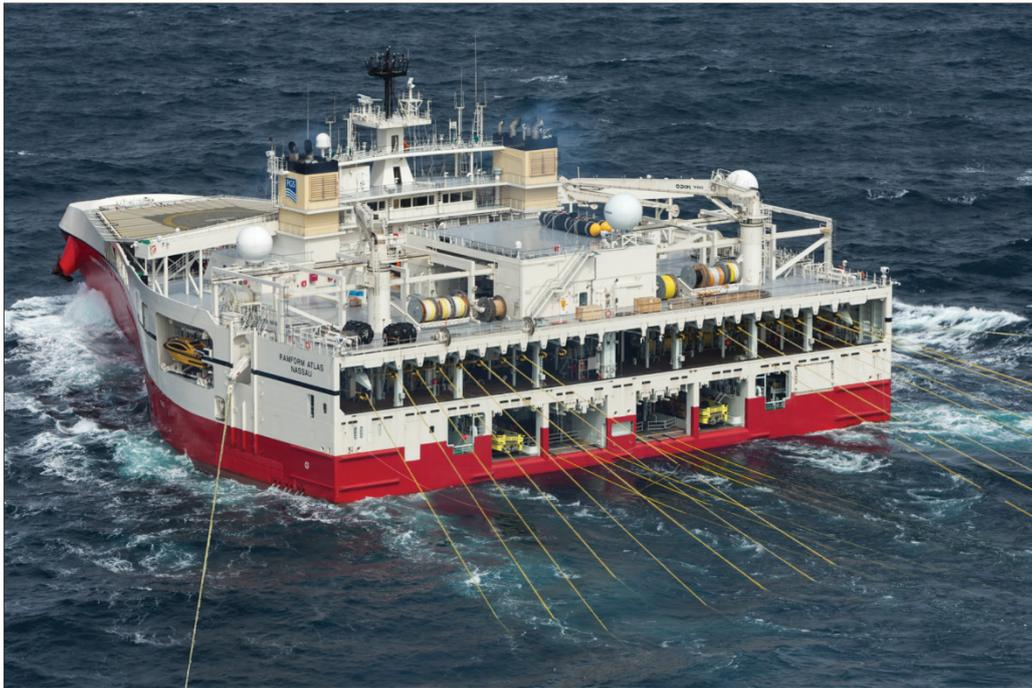
**Figure 3.2. Example of a modern marine setup for large-scale 3D seismic data collection.** The image depicts the *Ramform Atlas*, a 104 m long, 70 m wide seismic survey vessel owned by the marine geophysical company Petroleum Geo-Services (PGS). The survey vessel is capable of towing up to 24 streamer reels, allowing it to gather up to 200 km<sup>2</sup> of data in a single day (Jakobsson *et al.*, 2016). Photograph courtesy of PGS.
