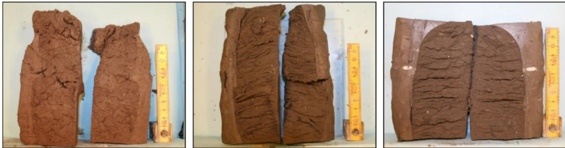
**Figure 8.3.** Examples of borehole samples recovered from the North Sea by the hydrocarbon industry after triaxial geotechnical testing. Similar samples have been recovered from inside tunnel valleys in the North Sea. The sample number and references to the sample owner have been removed for confidentiality purposes. The yellow ruler is 0.12 m high for scale.
