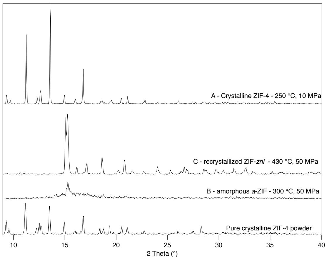
**Figure S1.** Powder X-ray diffraction patterns from crushed portions of sintered monoliths for phase identification and pure ZIF-4 powder.
