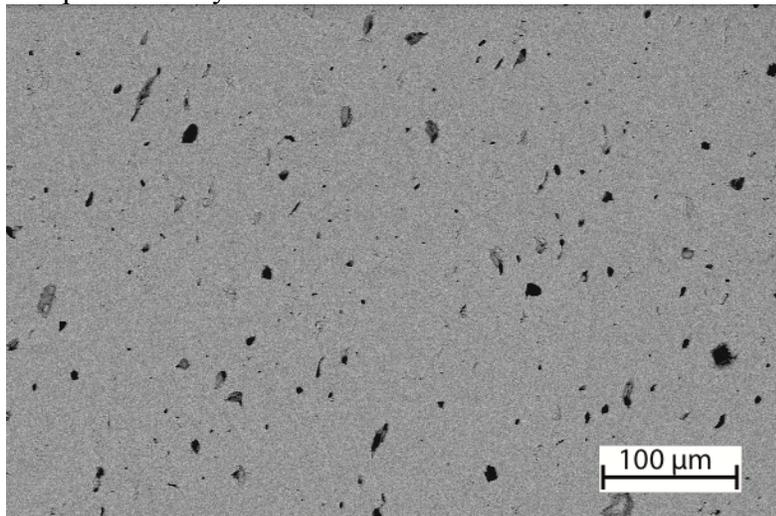
**Figure S3.** SEM images of Samples B and C. Backscattered electron images were recorded on polished surfaces. **Sample B:** Collapse of the crystallinity and softening of the grains supporting the originally highly porous microstructure lead to an almost fully densified microstructure. **Sample C:** recrystallization to ZIF-*zni* from amorphous *a*-ZIF entails a density increase, i.e. volume decrease, that could be responsible for the formation of isolated porosity (black spots).
