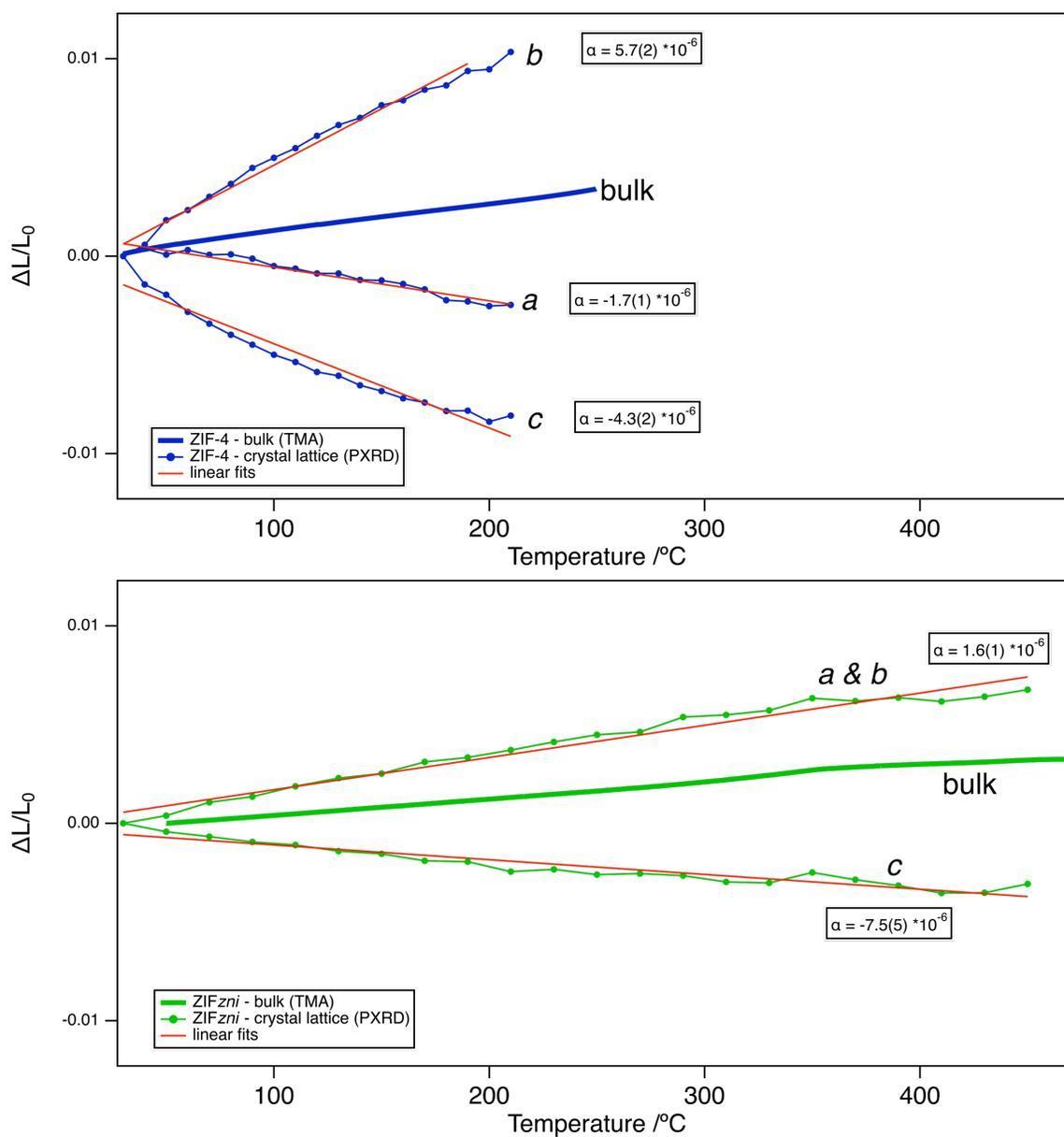
**Figure S5.** Temperature dependent relative unit cell dimensions of ZIF-4 (top) and ZIF-*zni* (bottom). ZIF-*zni* was prepared by heating ZIF-4 to 400 °C under vacuum (heating rate 0.5 °C/min). Thermal expansion coefficients  $\alpha$  derived from the slope of the linear fits (red lines).
