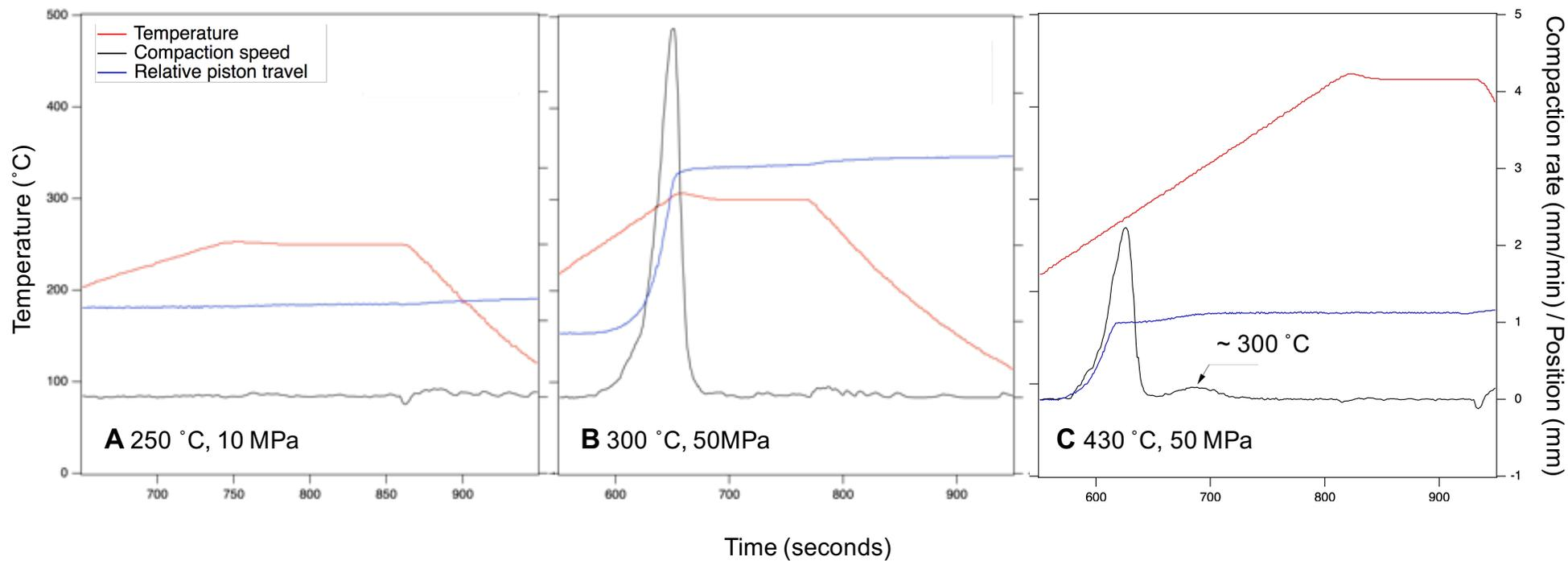
**Figure S4.** Sintering log data from individual runs. (A) Target temperature 250 °C and pressure 10 MPa, (B) target temperature 300 °C and pressure 50 MPa, (C) target temperature 430 °C and pressure 50 MPa.
