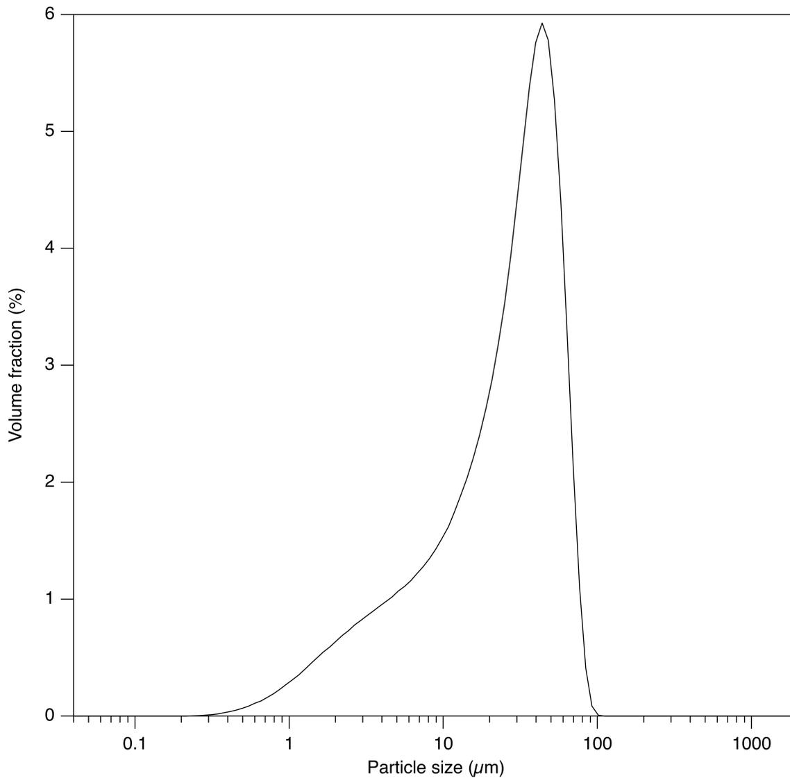
**Figure S2.** Particle size distribution of starting powder measured by Laser diffraction.
