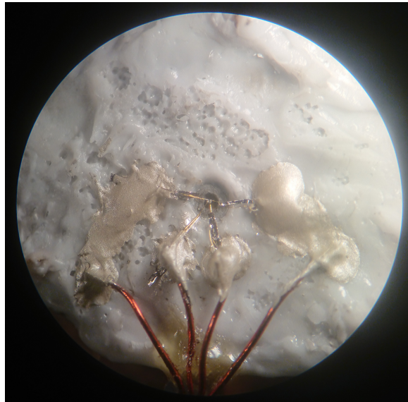
Fig. 4.19 A sample of antimony in the pressure cell with insulating gasket. The size of the sample is approximately 80\mu\text{m} \times 80\mu\text{m} \times 20\mu\text{m} and the size of the hole is 300\mu\text{m}
