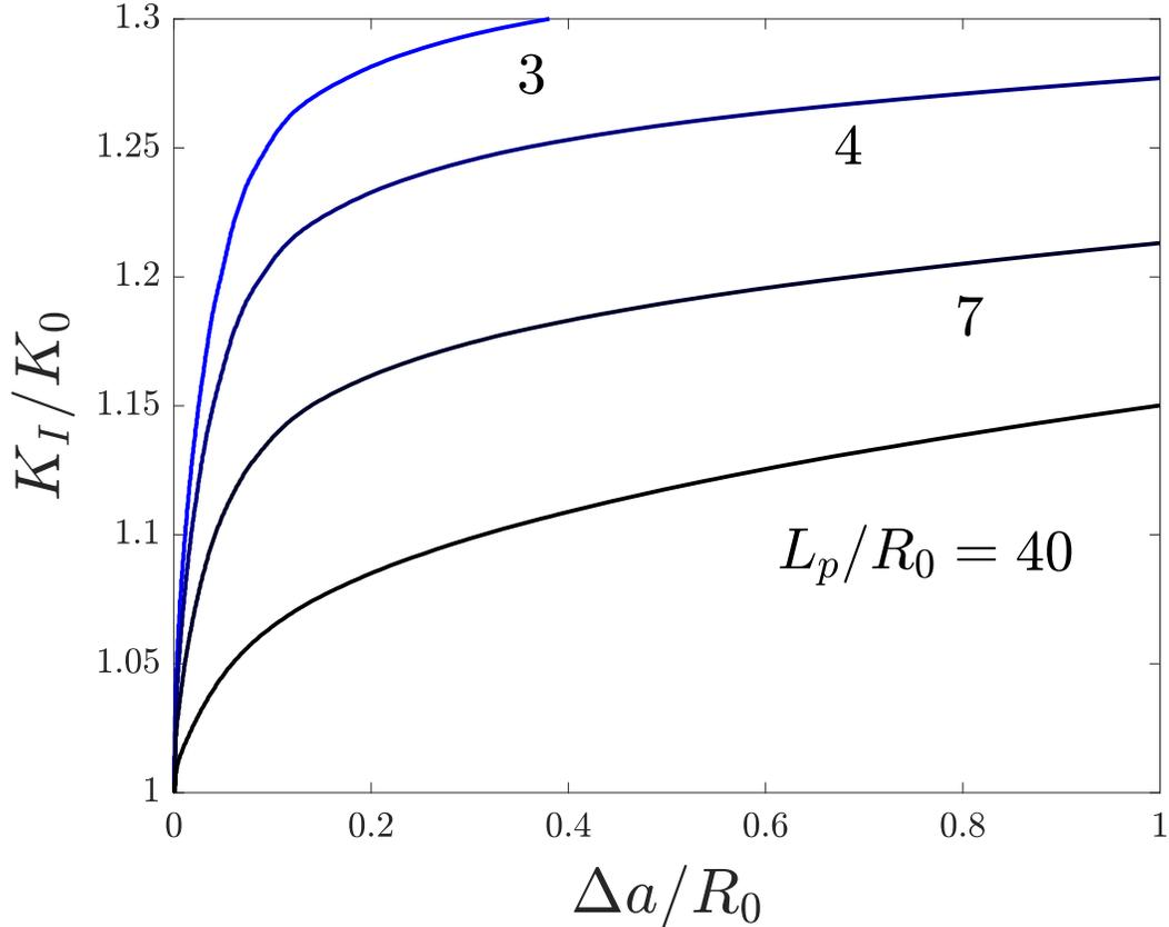
Figure 5: Influence of the plastic length scale ( $L_p$ ) on crack growth resistance. Material properties:  $\hat{\sigma}/\sigma_y \approx 6$  ( $\ell/R_0 = 1/40$ ),  $\sigma_y/E = 0.003$ ,  $\nu = 0.3$ ,  $N = 0.2$ .
