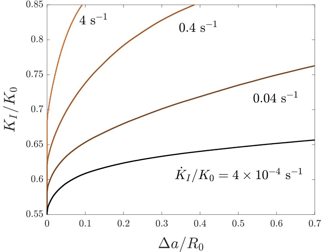
Figure 8: Effect of the loading rate ( $\dot{K}_I/K_0$ ) on the fracture resistance of samples pre-charged with a uniform hydrogen concentration of 0.5 wt ppm. Material properties:  $\sigma_y/E = 0.003$ ,  $\nu = 0.3$ ,  $N = 0.2$ ,  $\hat{\sigma}/\sigma_y \approx 6$  ( $\ell/R_0 = 0.025$ ),  $L_p/R_0 = 5$ ,  $D = 0.0127$  mm<sup>2</sup>/s, and  $\chi = 0.89$ .
