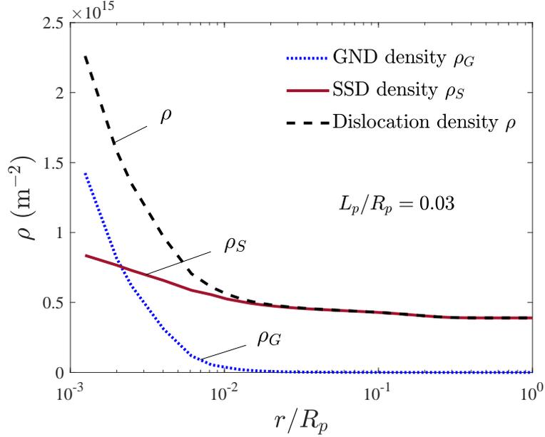
Figure 3: Stationary crack tip analysis: dislocation density distribution (in  $\text{m}^{-2}$ ) ahead of the crack ( $r, \theta = 0^\circ$ ). Results are shown for  $L_p/R_p = 0.03$ , presenting the distribution of the GND dislocation density  $\rho_G$ , the SSD dislocation density  $\rho_S$  and the total dislocation density  $\rho$ .
