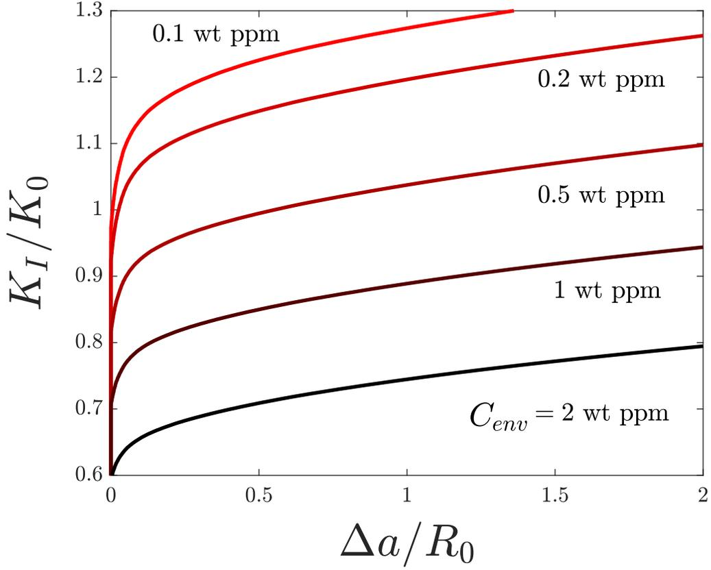
Figure 7: Effect of the environmental hydrogen concentration on the fracture resistance. Material properties:  $\sigma_y/E = 0.003$ ,  $\nu = 0.3$ ,  $N = 0.2$ ,  $\hat{\sigma}/\sigma_y = 10$  ( $\ell/R_0 = 1/110$ ),  $L_p/R_0 = 5$ ,  $D = 0.0127 \text{ mm}^2/\text{s}$ , and  $\chi = 0.89$ . Loading rate  $\dot{K}_I/K_0 = 4 \times 10^{-7} \text{ s}^{-1}$ .
