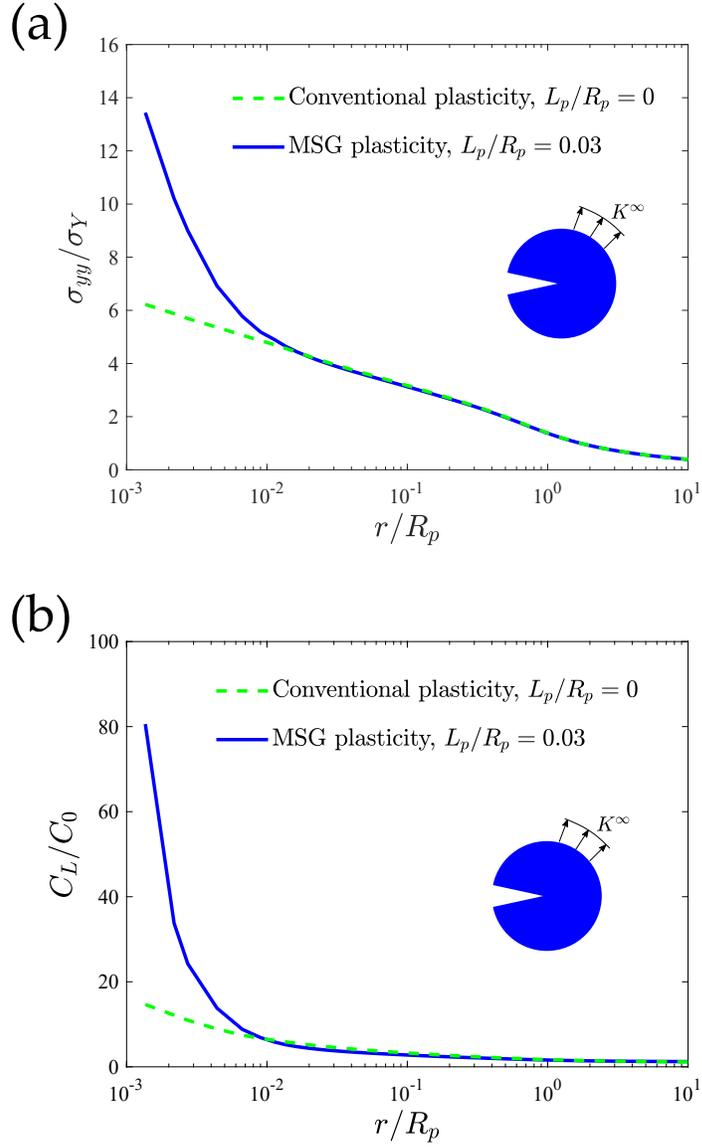
Figure 2: Stationary crack tip analysis: (a) tensile stress and (b) lattice hydrogen concentration distributions ahead of the crack ( $r, \theta = 0^\circ$ ). Results are shown for both mechanism-based strain gradient (MSG) plasticity ( $L_p/R_p = 0.03$ ) and conventional plasticity ( $L_p/R_p = 0$ ).
