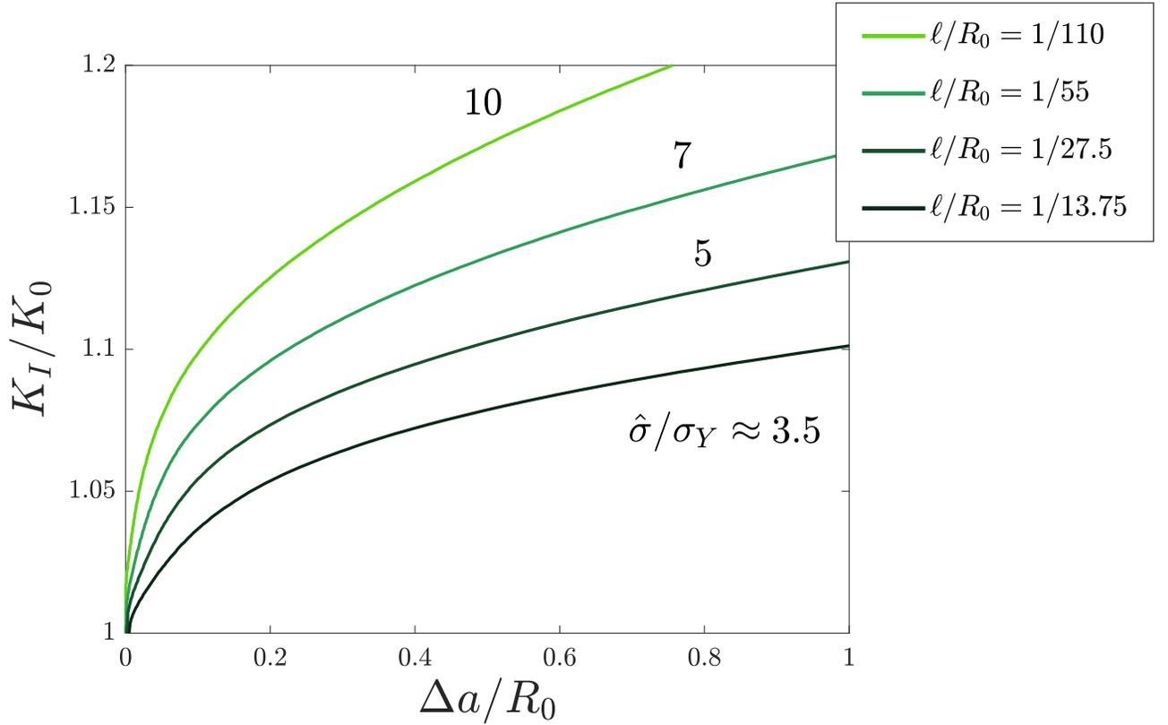
Figure 6: Influence of the material strength  $\hat{\sigma}/\sigma_Y$  ( $\ell/R_0$ ) on crack growth resistance. Material properties:  $\sigma_Y/E = 0.003$ ,  $\nu = 0.3$ ,  $N = 0.2$ , and  $L_p/R_0 = 40$ .
