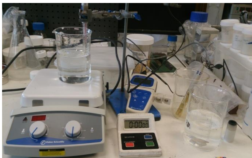
Figure 3.2 Set up for the reactivity test of MgO.
