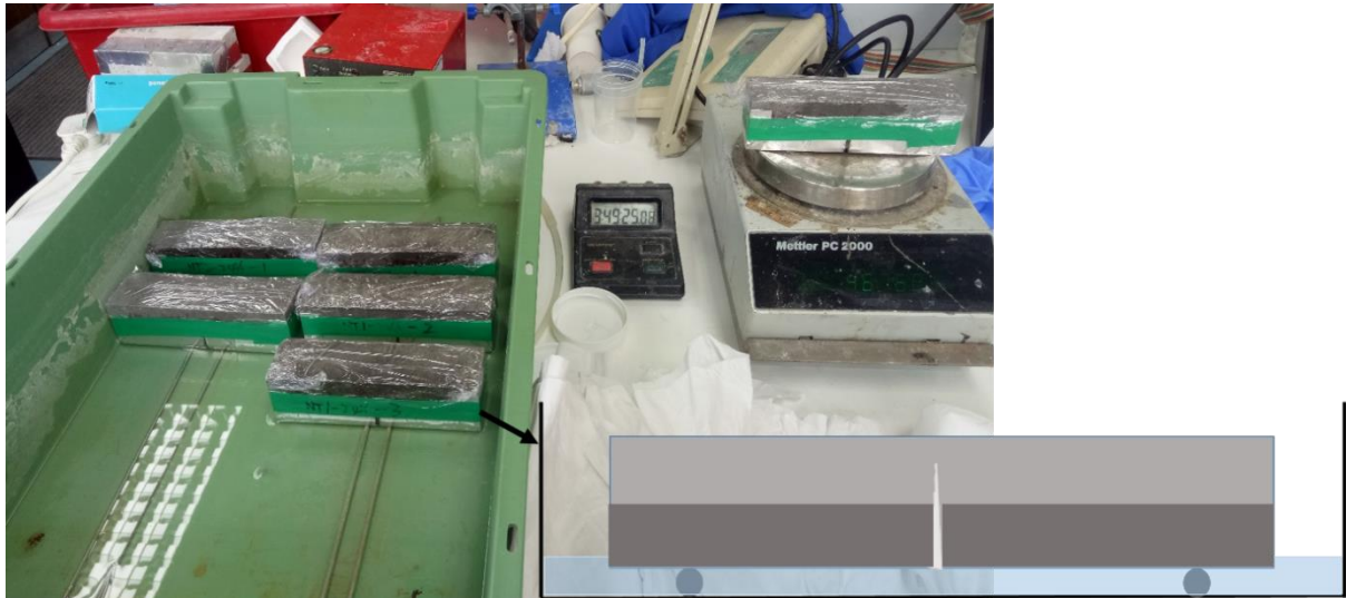
Figure 3.20 Illustration of the capillary water absorption testing procedure.
