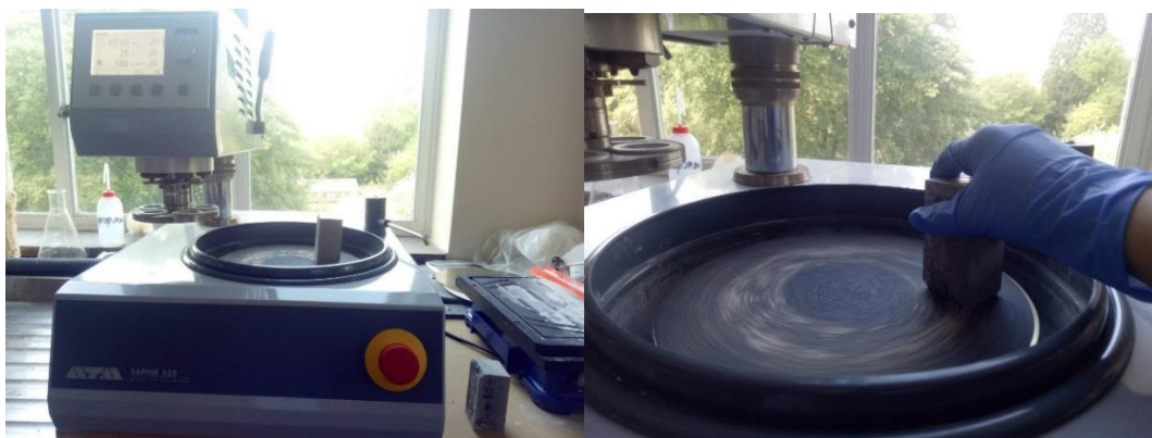
Figure 3.23 Powder sample extraction from the crack surface of cement prisms containing microcapsules.
