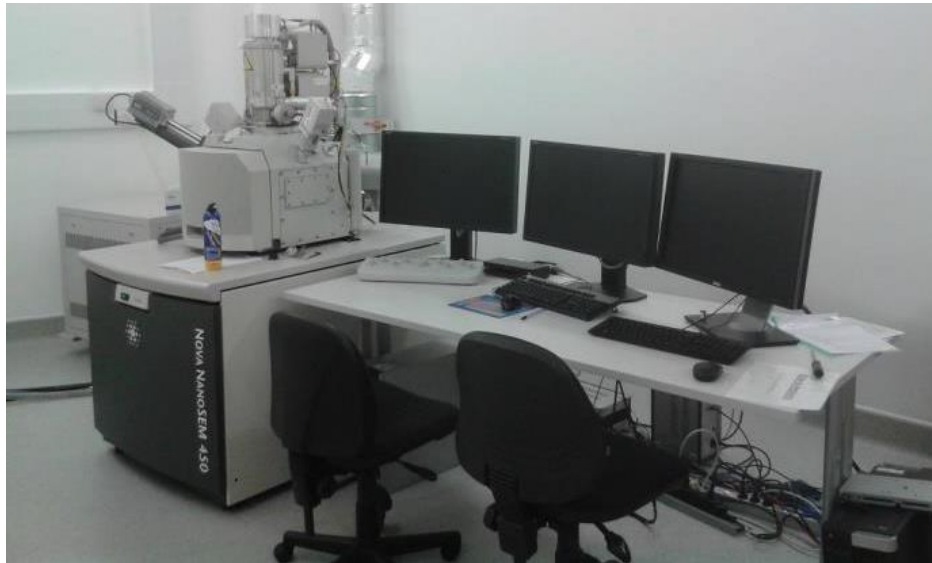
Figure 3.25 FEI Nova NanoSEM FEG for characterisation on MgO hydration products as well as self-healing products of sodium silicate microcapsules in cement pastes.
