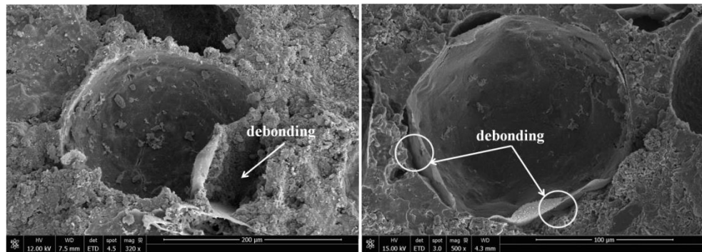
Figure 5.7 SEM images of microcapsule shells debonded from the surrounding cement matrix
