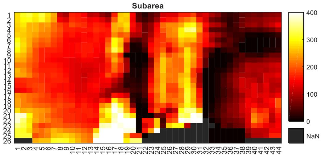
Figure 13: Filtered data for slab-soil contact pressure, extracted by filtering the data in Figure 11
