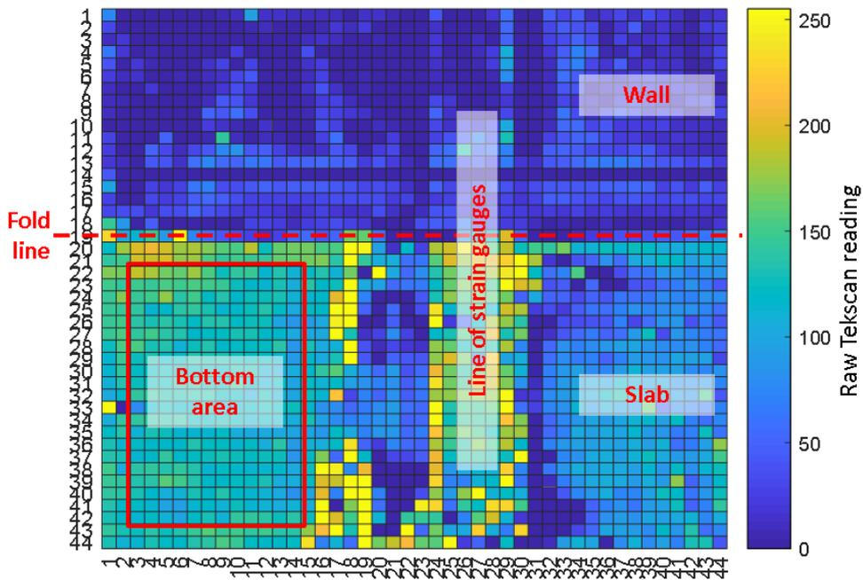
Figure 8: Illustration of the different regions measured by the tactile sensing mat, using the "slab" mat from centrifuge test *DYC-06* as an example
