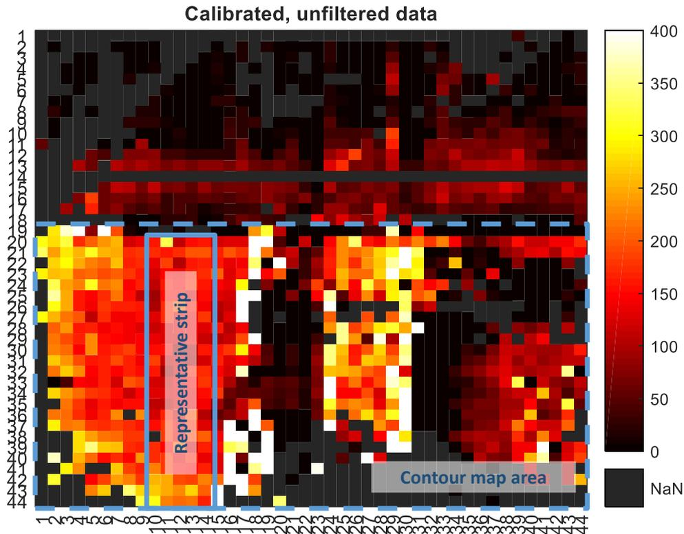
Figure 11: Calibrated, unfiltered heat map plot of data from equilibrium slab-soil contact pressure in centrifuge test *DYC-06*, to illustrate the process of filtering and contouring
