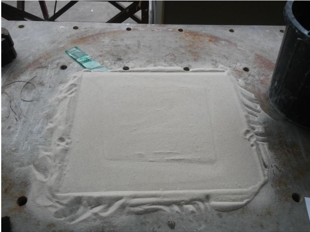
*Figure 4: Tekscan sheet buried between hydraulic jack platform and Hostun sand layer*
