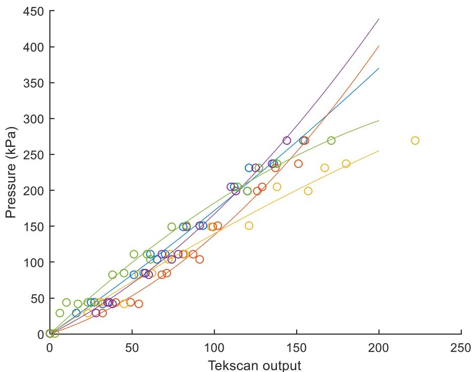
Figure 5: Plot of the responses of five randomly selected sensels from the calibration used in centrifuge test *DYC-06*. Curved lines are quadratic best-fits.
