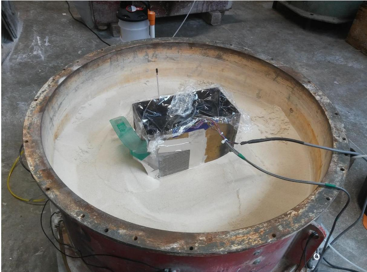
Figure 2: Basement model with Tekscan sheet installed into centrifuge package, during the preparation of centrifuge test DYC-03
