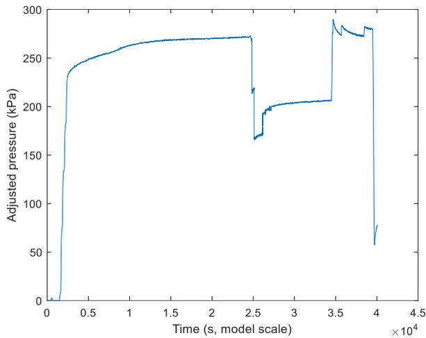
Figure 10: Adjusted average slab-soil contact pressure, centrifuge test DYC-06
