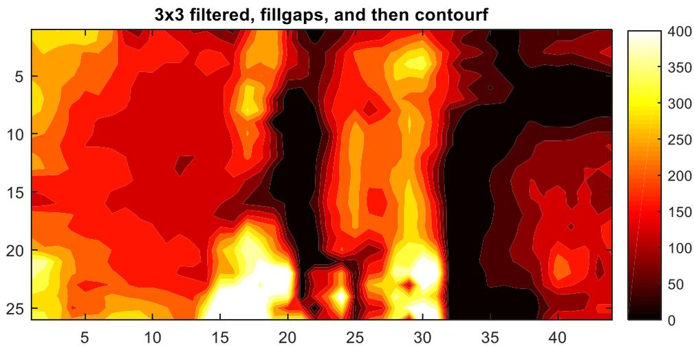
Figure 14: Contour plot of slab-soil contact pressure
