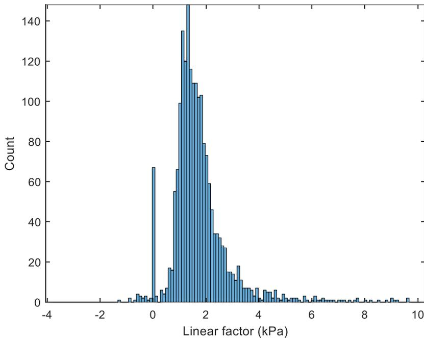
Figure 6: Histogram of linear factors, from slab Tekscan sheet in test DYC-06
