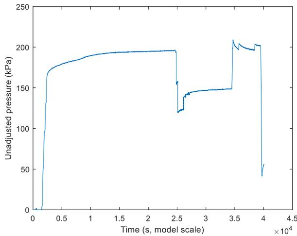
Figure 9: Variation with time of unadjusted pressure readings of slab-soil contact pressure on the non-edge regions, from centrifuge test *DYC-06*
