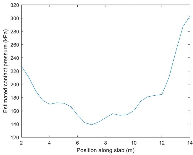
Figure 12: Plot of filtered pressure data along a representative strip
