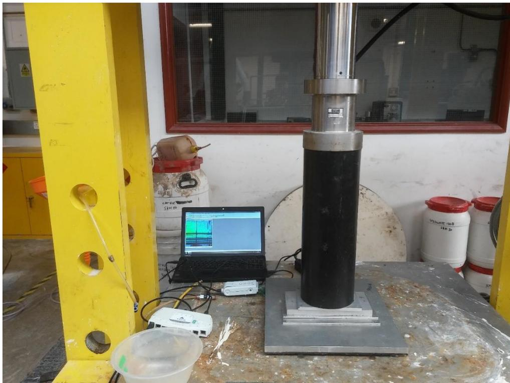
*Figure 3: Calibrating a Tekscan sheet by applying a known load through a hydraulic piston*
