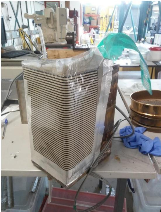
Figure 1: Tekscan sheet attached onto structural model for centrifuge test DYC-04
